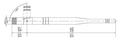
Figure 3-6 ZXT9-IO-222R2 Supplied Antenna
