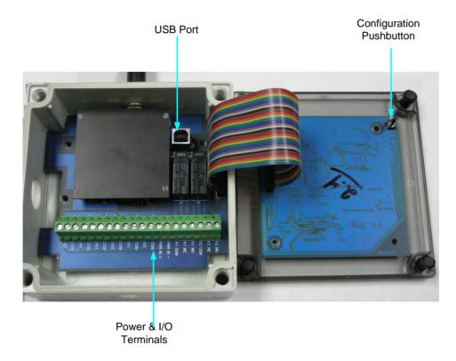
Figure 2-6 Internal View of Zlinx Xtreme I/O module
