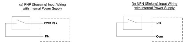
Figure 7-2 Digital Input (Sourcing driver) wiring
