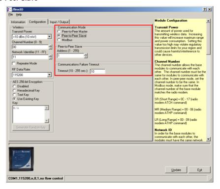
Fig 6-15 Peer-to-Peer Slave Configuration
