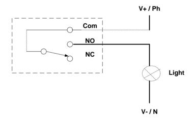
Figure 7-3 Relay Output Testing
