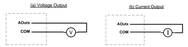
Figure 4-8 Typical Analog Output Wiring
