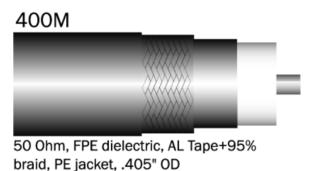
Figure 3-14 LMR400 Cable Cross Section
