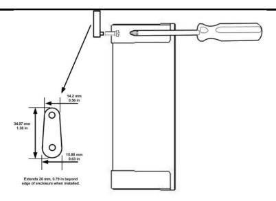
Figure 3-2 Mounting Ear dimensions
