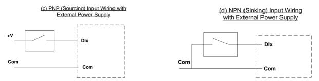
Figure 4-4 Typical Digital Input Wiring for PNP and NPN connection types (with external PS)
