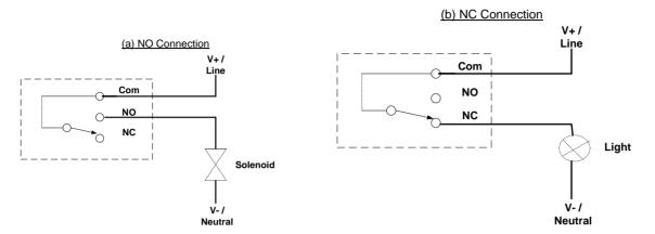
Figure 4-6 Typical Digital Output Wiring for Relay Outputs
