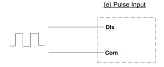
Figure 4-5 Pulse Input Connection
