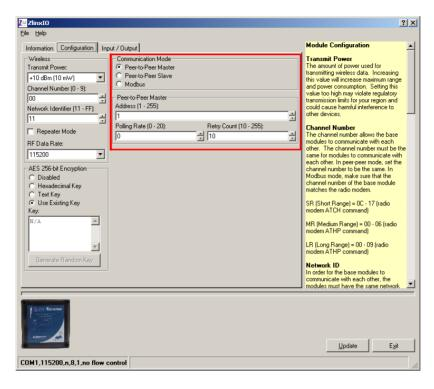
Fig 6-14 Peer-to-Peer Master Configuration
