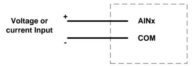
Figure 4-7 Typical Analog Input Wiring
