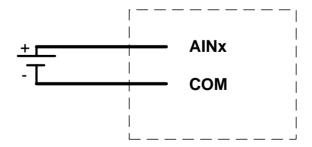
Figure 7-4 Analog Input wiring
