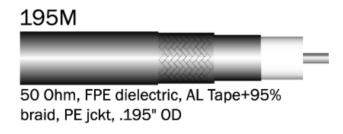
Figure 3-15 LMR195 Cable Cross Section
