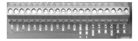
Figure 4-1 I/O Terminal Layout
