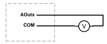
Figure 7-5 Analog Output (Sourcing driver) wiring
