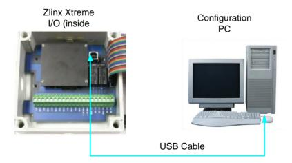
Figure 5-3 PC to I/O Module Connection
