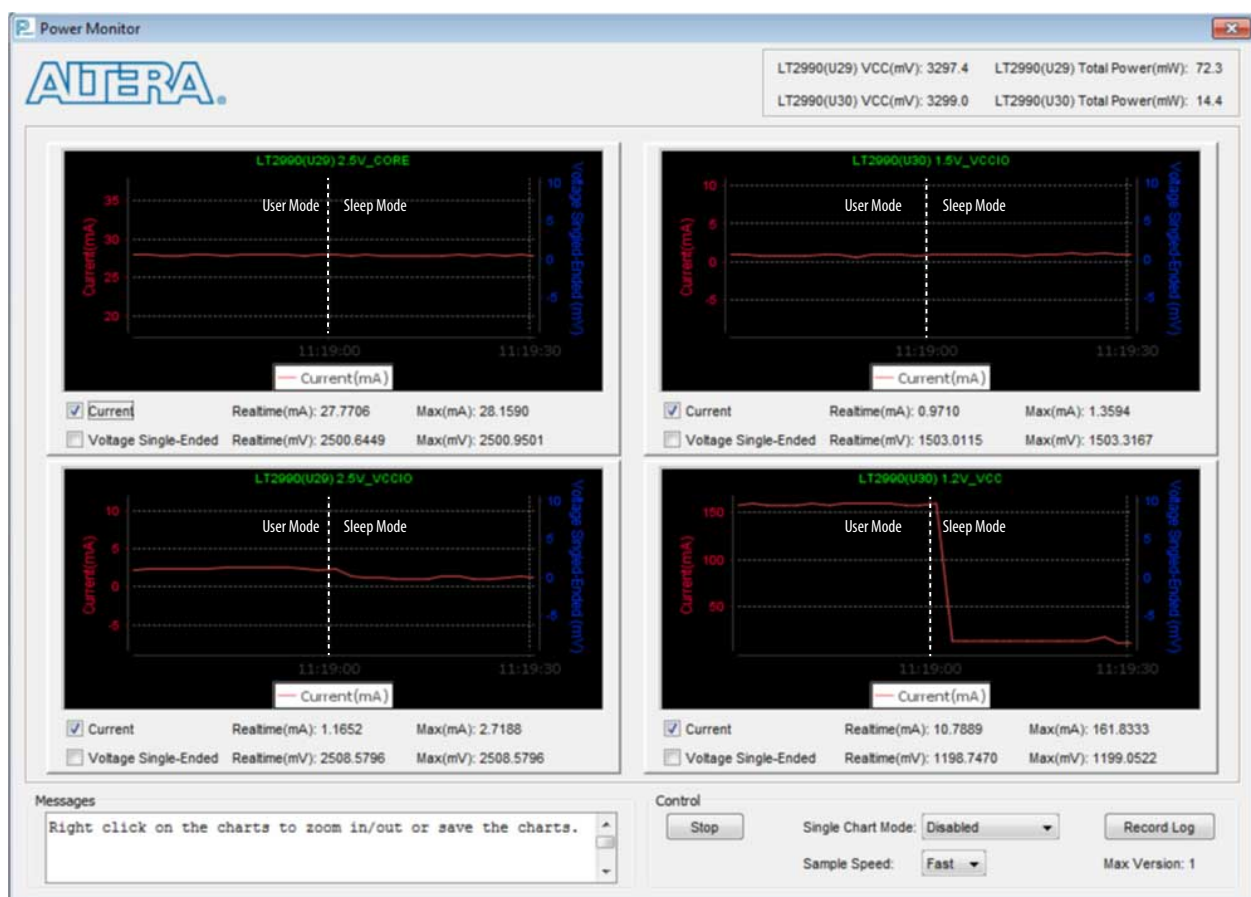
Figure 3-5: Current Monitor for Each Supply
