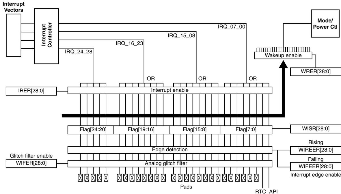
**Figure 12-12. External interrupt pad diagram**
