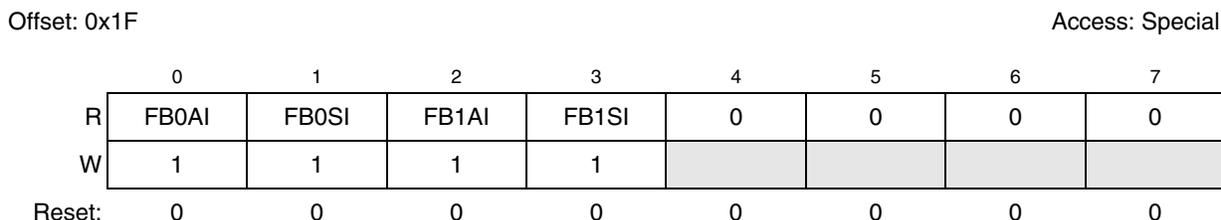
**Figure 34-5. Miscellaneous Interrupt (MIR) Register**
