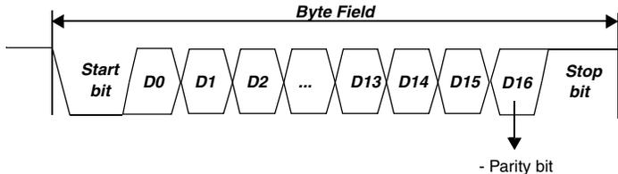
Figure 24-17. UART mode 17-bit data frame
