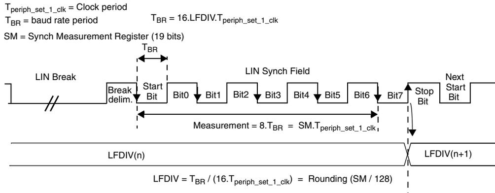
Figure 23-31. LIN synch field measurement
