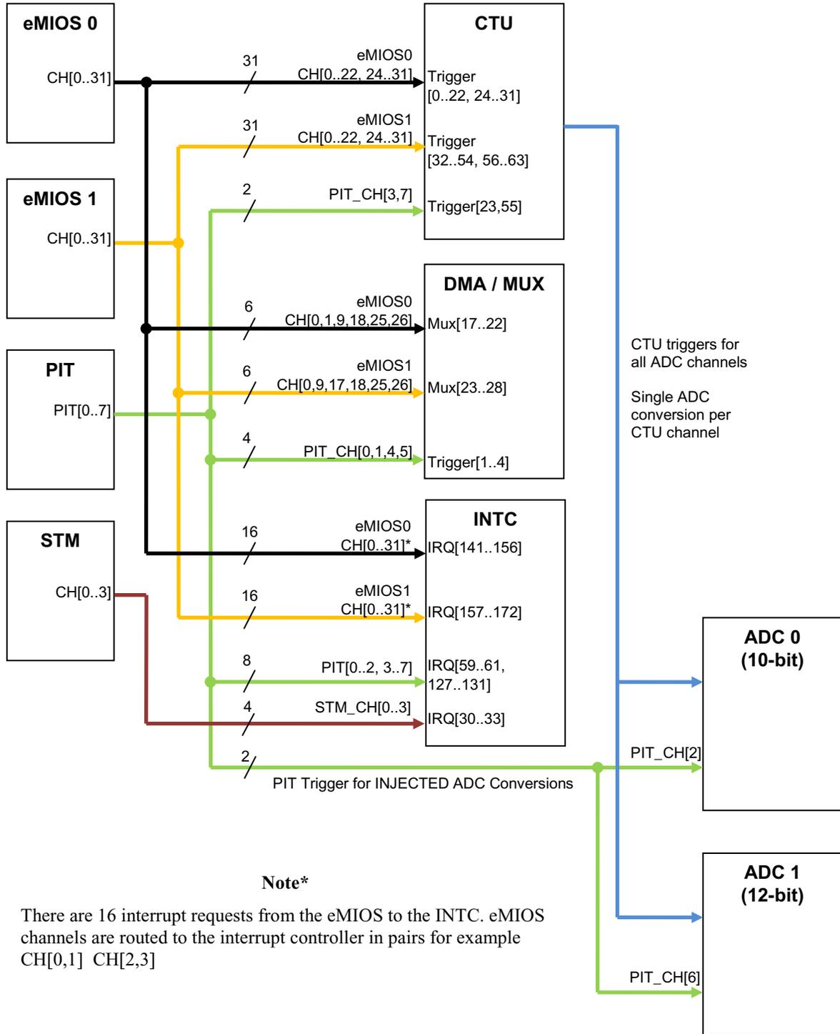
Figure 27-1. Interaction between timers and relevant peripherals
