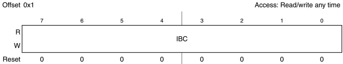
**Figure 22-3. I<sup>2</sup>C Bus Frequency Divider Register (IBFD)**
