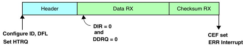
Figure 24-60. Programming consideration: master node, receiver, checksum error
