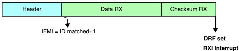
Figure 24-66. Programming consideration: slave node, at least one RX filter, BF is reset, ID matches filter
