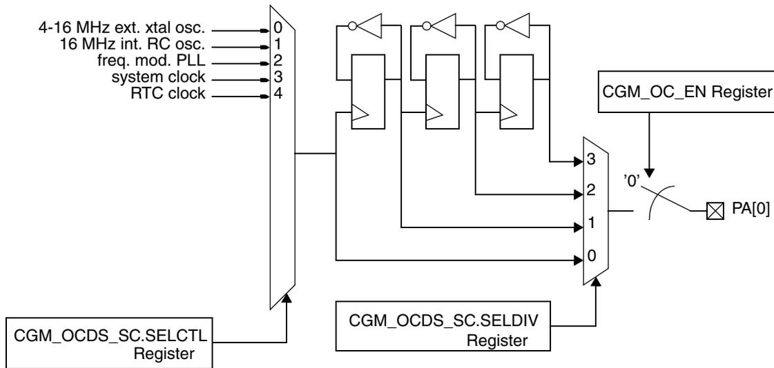
Figure 7-7. MC\_CGM Output Clock Multiplexer and PA[0] Generation
