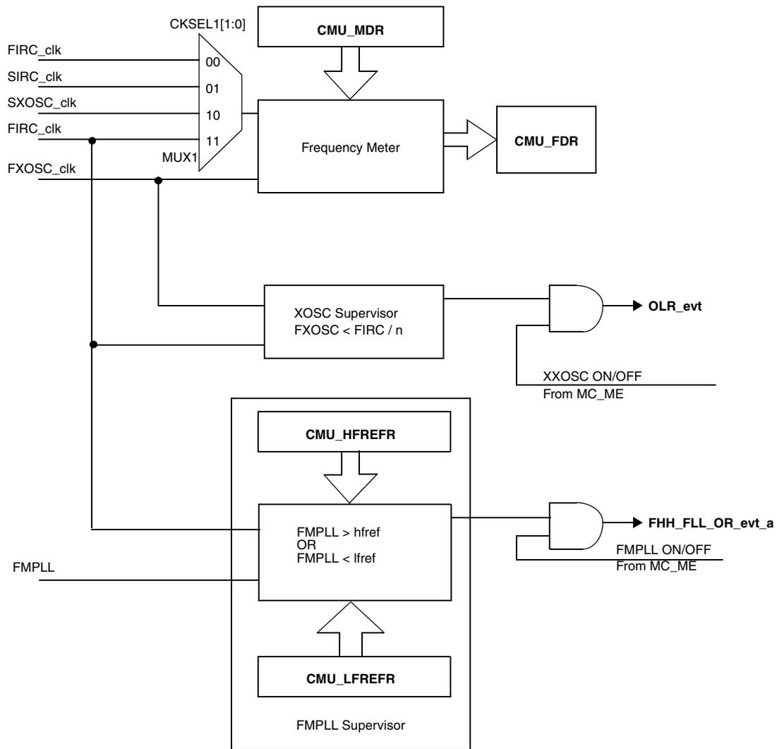
**OLR\_evt** : It is the event signalling XOSC failure when asserted. When this signal is asserted, RGM may generate reset, interrupt or SAFE request based on the RGM configuration.
