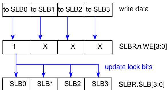
**Figure 32-7. Change Lock Settings for 32-bit Protected Addresses**
