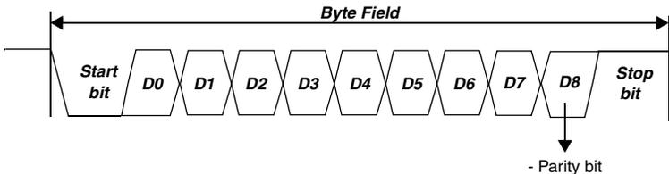
Figure 24-15. UART mode 9-bit data frame
