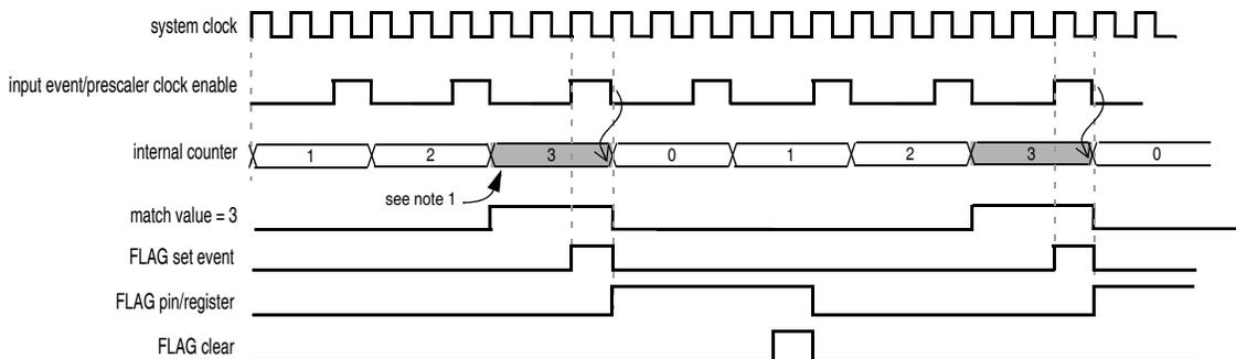
Note 1: The match occurs only when the input event/prescaler clock enable is active. Then, the internal counter is immediately cleared.
