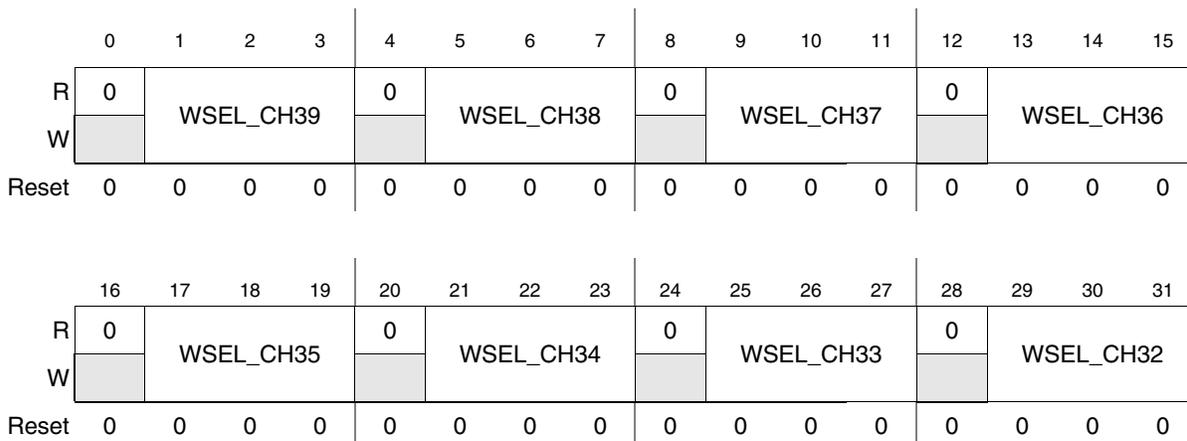
**Figure 28-52. Channel Watchdog Select Register 4 (CWSELR4) – ADC\_0**
