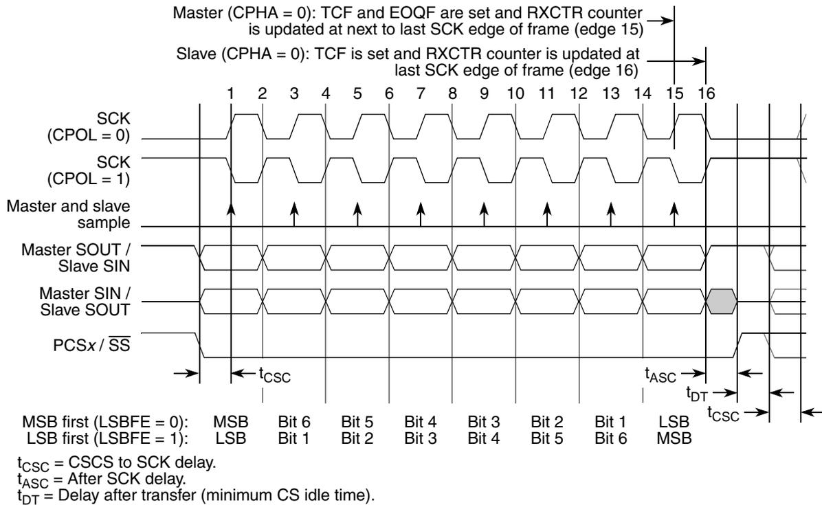
Figure 26-16. DSPI transfer timing diagram (MTFE = 0, CPHA = 0, FMSZ = 8)
