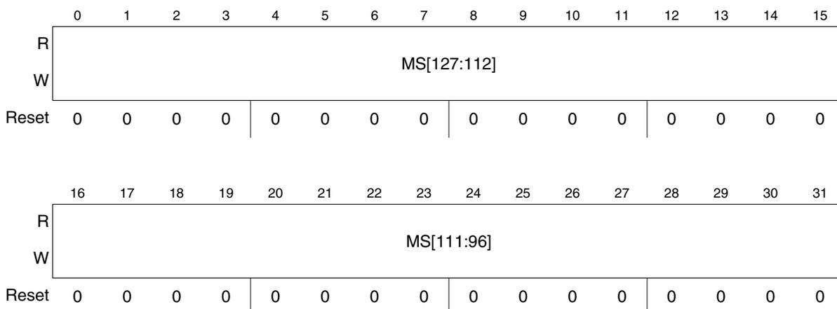
**Figure 30-19. CFlash User Multiple Input Signature Register 3 (CFLASH\_UMISR3)**
