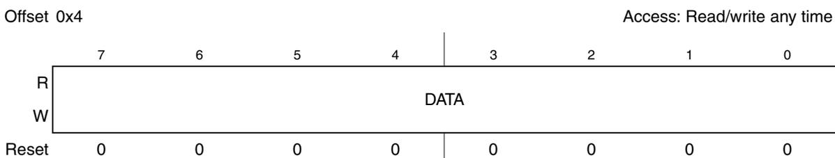
**Figure 22-8. I<sup>2</sup>C Bus Data I/O Register (IBDR)**
