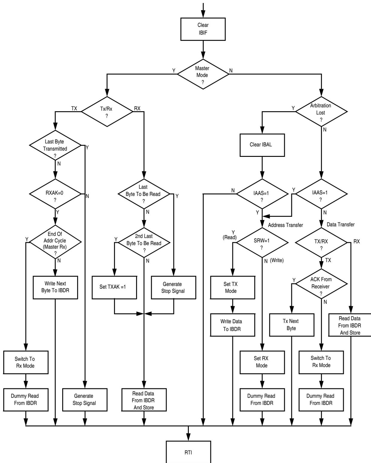
Figure 22-14. Flow-Chart of Typical I<sup>2</sup>C Interrupt Routine
