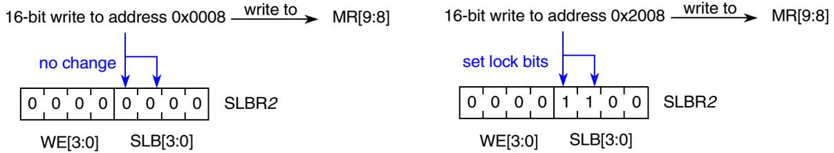
**Figure 32-9. Enable Locking Via Mirror Module Space (Area #3)**
