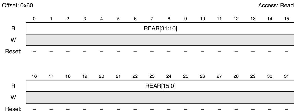
Figure 34-14. Platform RAM ECC Address Register (PREAR)
