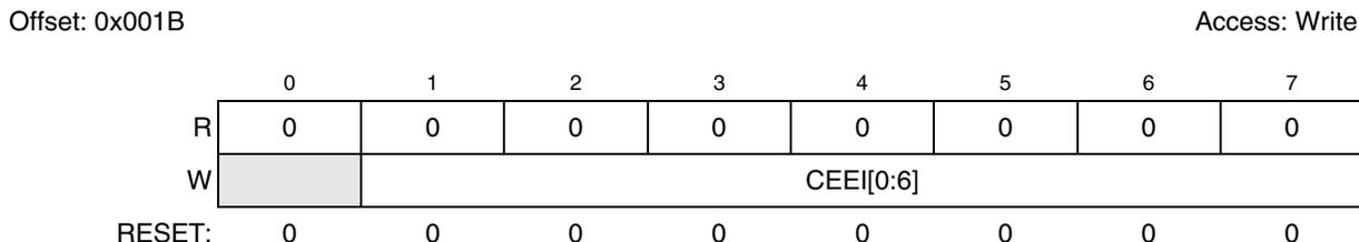
**Figure 16-9. DMA Clear Enable Error Interrupt (EDMA\_CEEIR) Register**
