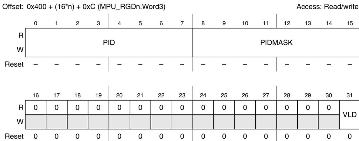
**Figure 20-8. MPU Region Descriptor, Word 3 Register (MPU\_RGDn.Word3)**
