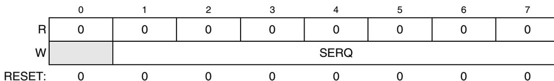
Figure 16-6. DMA Set Enable Request (EDMA\_SERQR) Register
