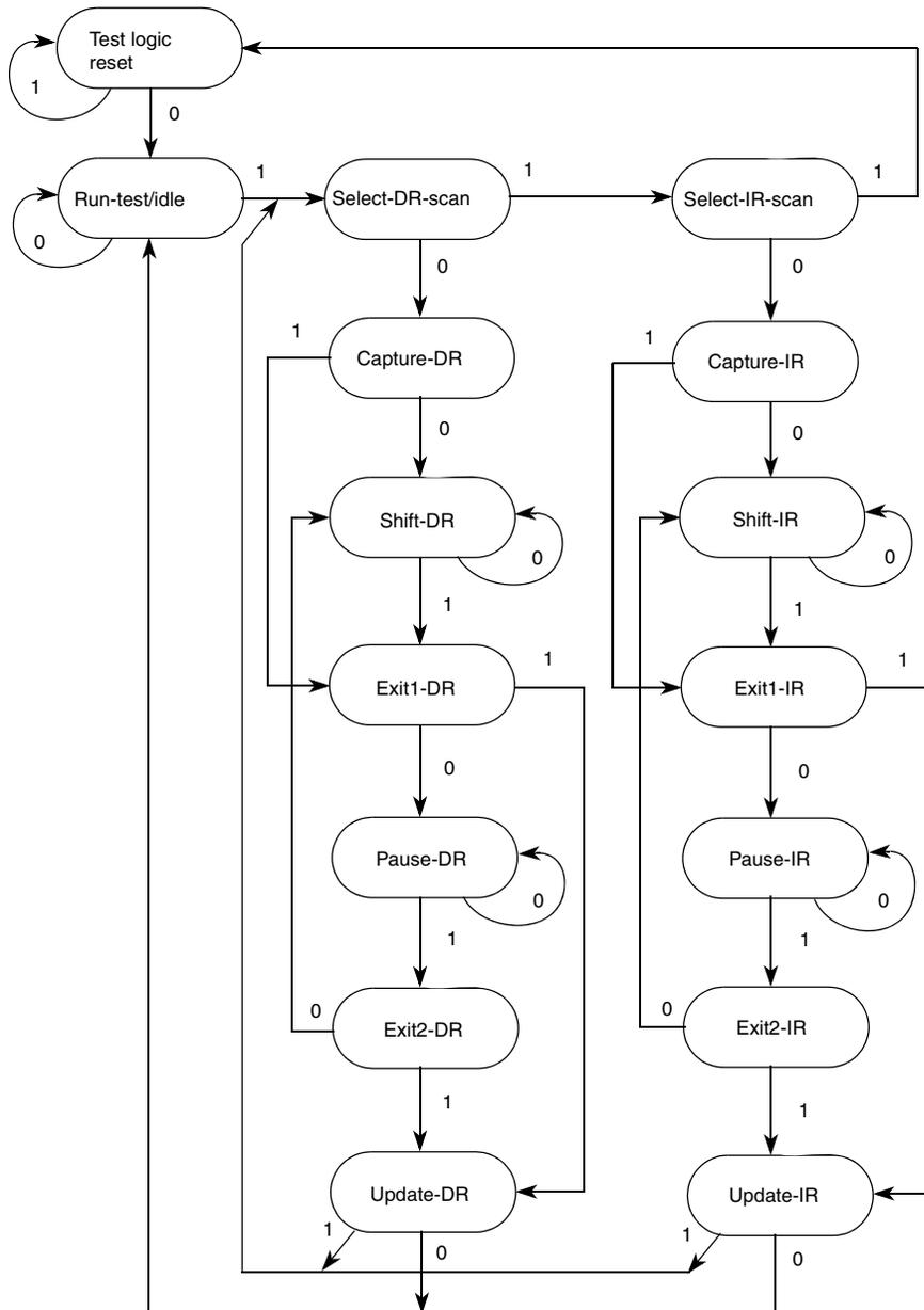
NOTE: The value shown adjacent to each state transition in this figure represents the value of TMS at the time of a rising edge of TCK.
