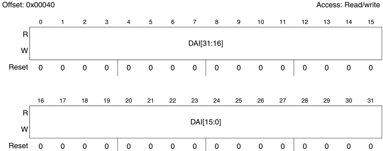
**Figure 30-14. CFlash User Test 1 register (CFLASH\_UT1)**
