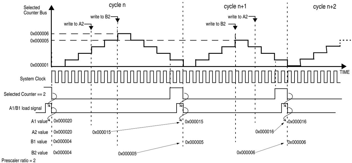
**Figure 27-40. OPWMCB A1 and B1 registers load**
