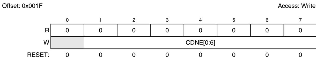
**Figure 16-13. DMA Clear DONE Status (EDMA\_CDSBR) Register**
