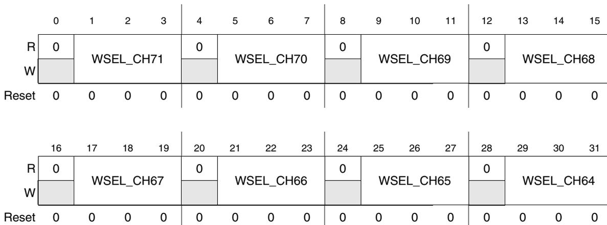
**Figure 28-56. Channel Watchdog Select Register 8 (CWSELR8) – ADC\_0**
