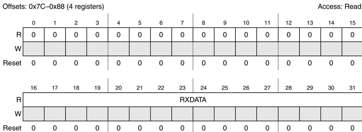
Figure 26-11. DSPI Receive FIFO Registers 0–3 (DSPIx\_RXFRn)
