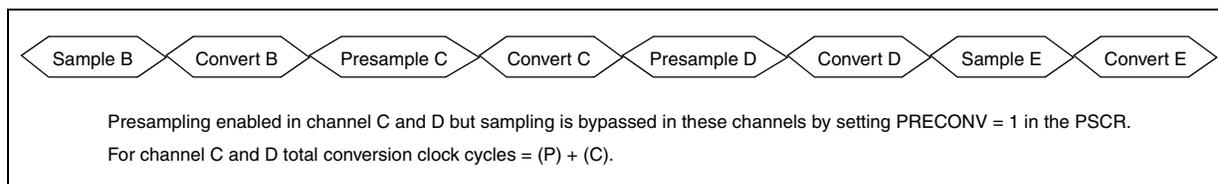
Figure 28-7. Presampling sequence with PRECONV = 1
