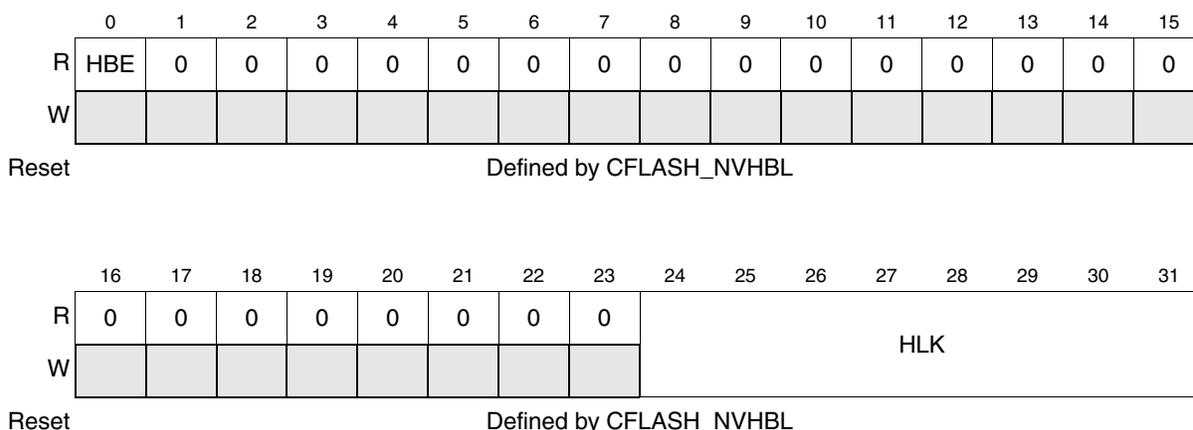
**Figure 30-6. CFlash Nonvolatile High Address Space Block Locking Register (CFLASH\_HBL)**
