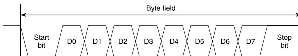
Figure 5-10. LINFlex bit timing in UART mode
