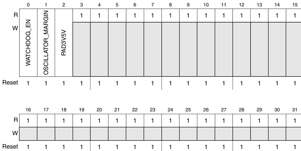
Figure 30-25. CFlash Nonvolatile User Options register (NVUSRO)
