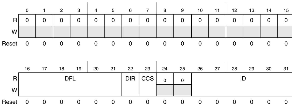
**Figure 24-31. Buffer identifier register (BIDR)**
