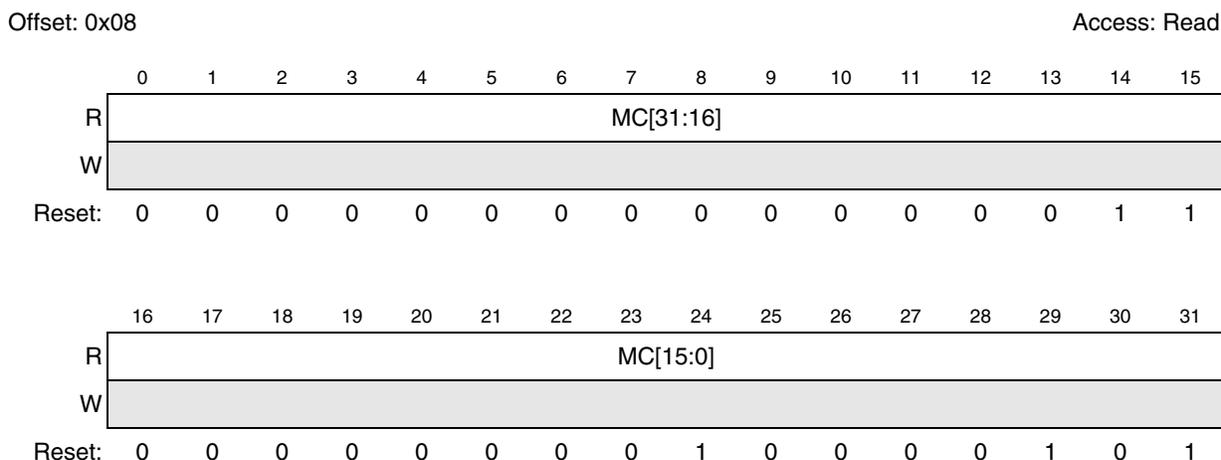
**Figure 34-3. IPS On-Platform Module Configuration Register (IOPMC)**
