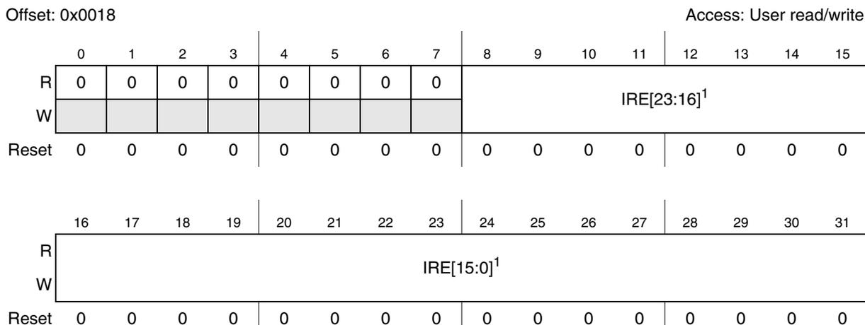
**Figure 21-5. Interrupt Request Enable Register (IRER)**
