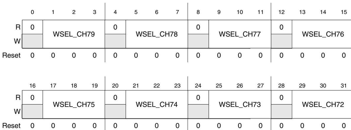
**Figure 28-57. Channel Watchdog Select Register 9 (CWSELR9) – ADC\_0**
