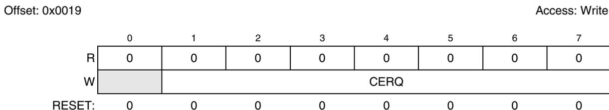
**Figure 16-7. DMA Clear Enable Request (EDMA\_CERQR) Register**
