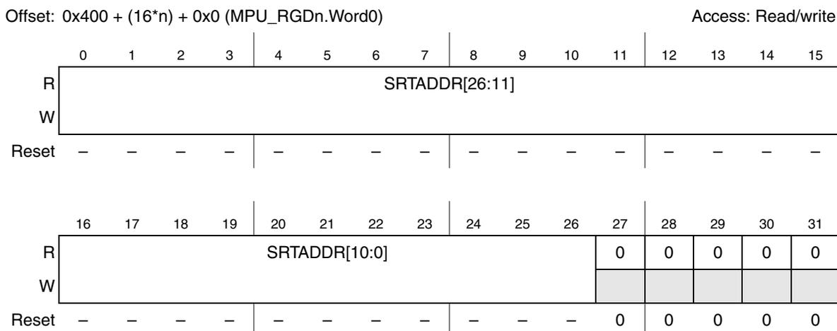
**Figure 20-5. MPU Region Descriptor, Word 0 Register (MPU\_RGDn.Word0)**
