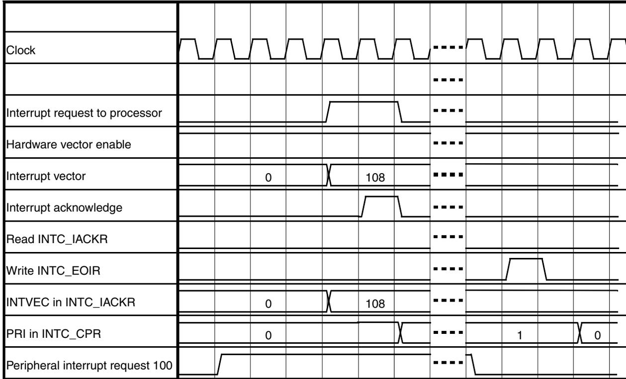
Figure 18-12. Hardware vector mode handshaking timing diagram
