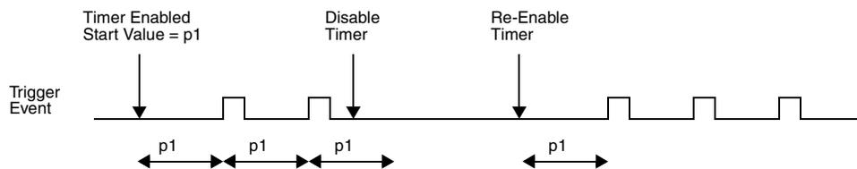
**Figure 27-62. Stopping and starting a timer**
