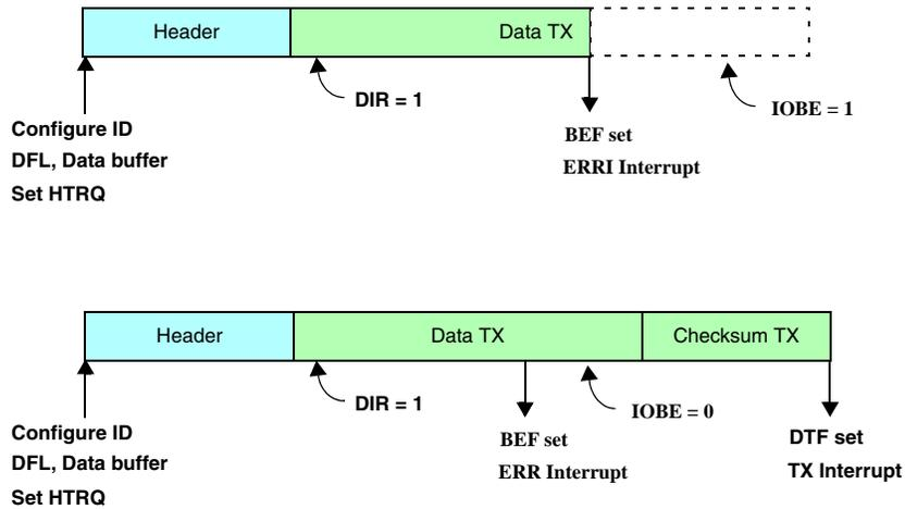
Figure 24-59. Programming consideration: master node, transmitter, bit error
