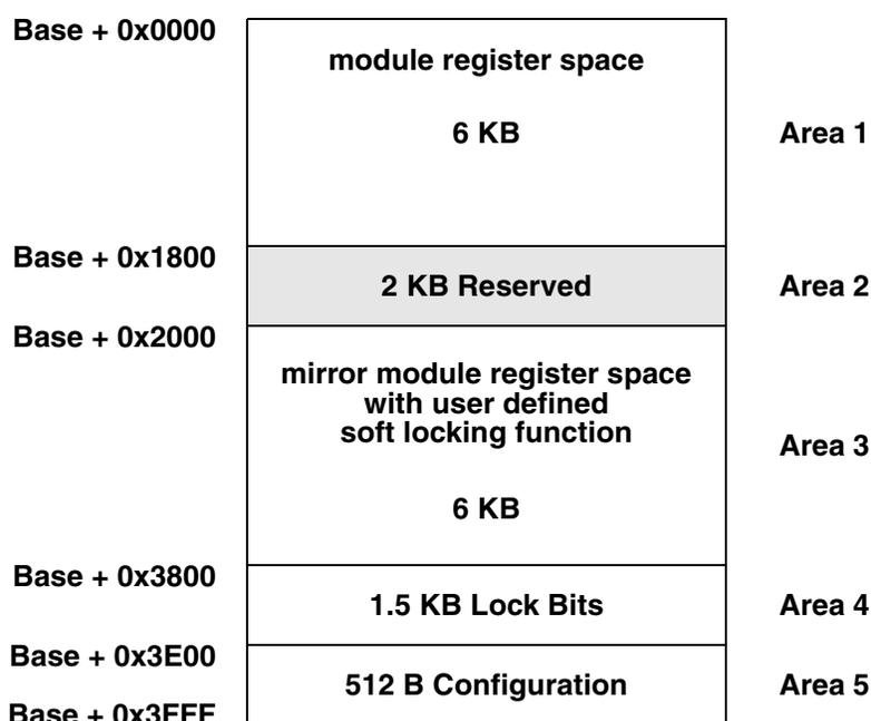
**Figure 32-2. Register protection memory diagram**
