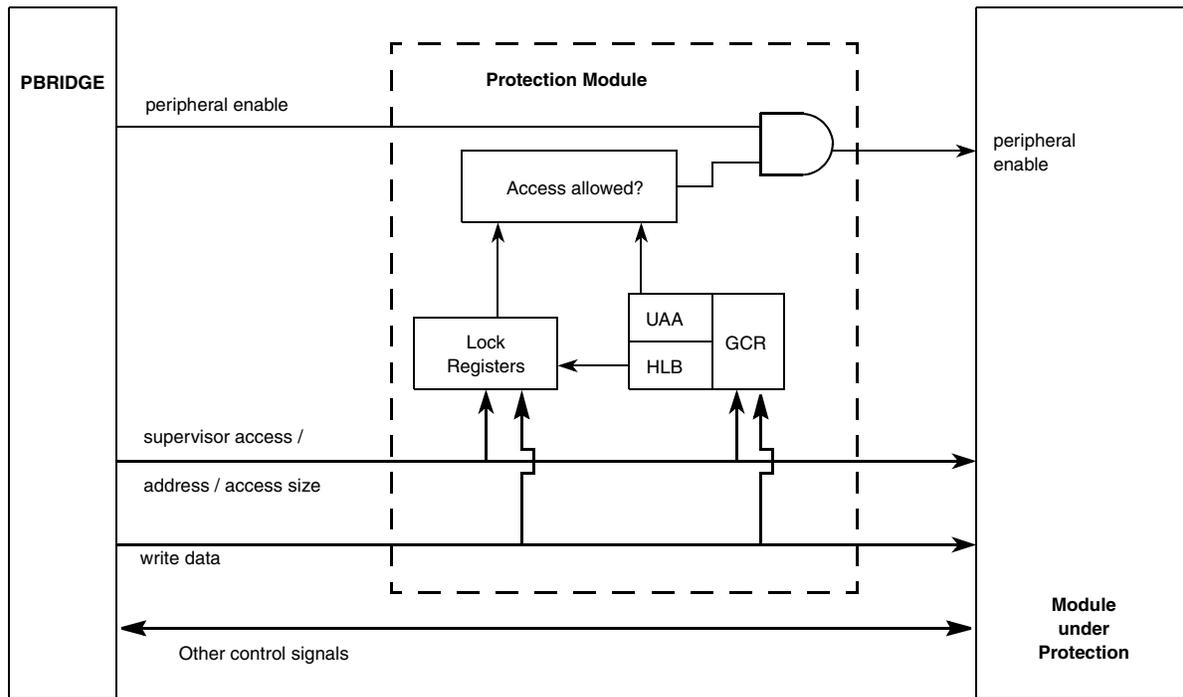
**Figure 32-1. Register Protection block diagram**
