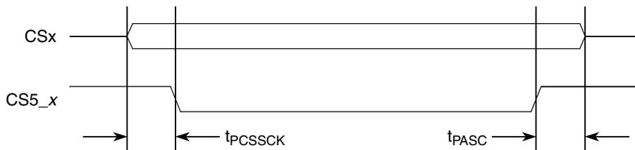
**Figure 26-15. Peripheral chip select strobe timing**
