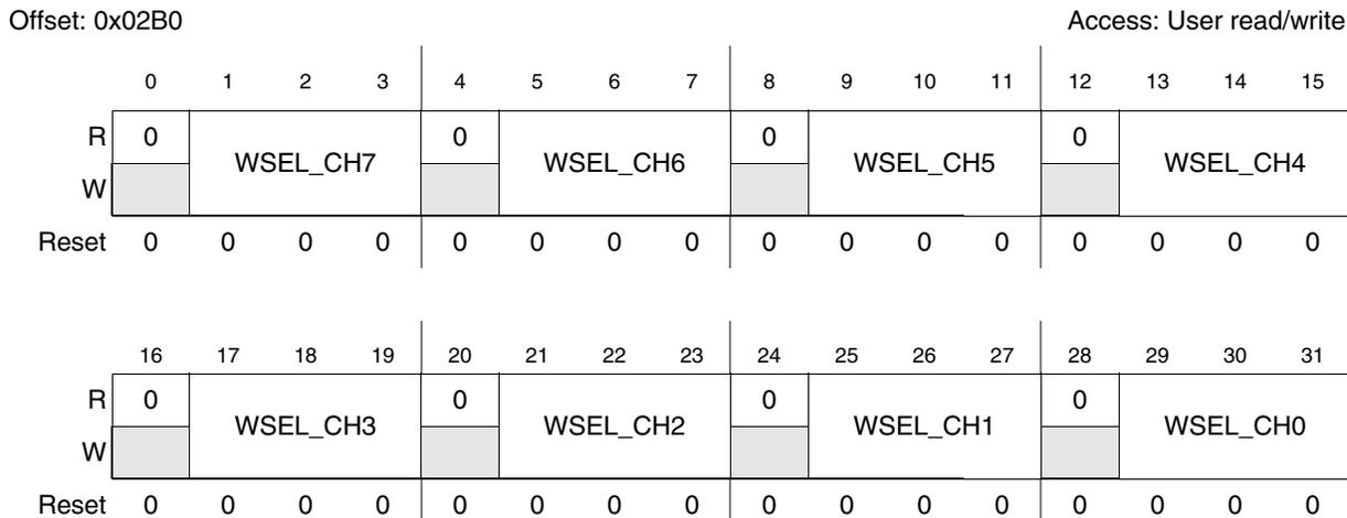
**Figure 28-50. Channel Watchdog Select Register 0 (CWSELR0) – ADC\_0**
