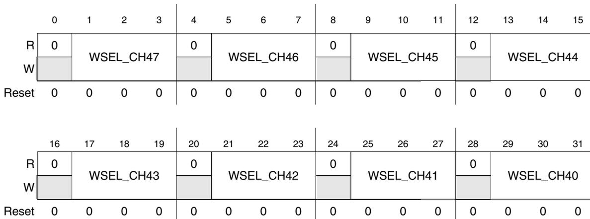
**Figure 28-53. Channel Watchdog Select Register 5 (CWSELR5) – ADC\_0**
