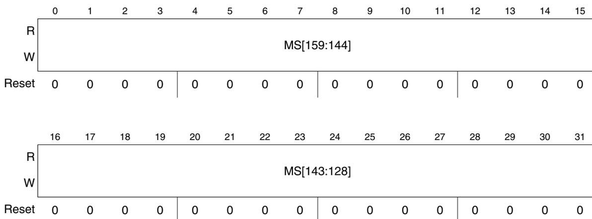
**Figure 30-20. CFlash User Multiple Input Signature Register 4 (CFLASH\_UMISR4)**
