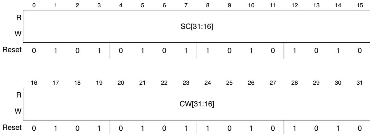
**Figure 30-24. CFlash Nonvolatile System Censorship Control 1 register (NVSCC1)**
