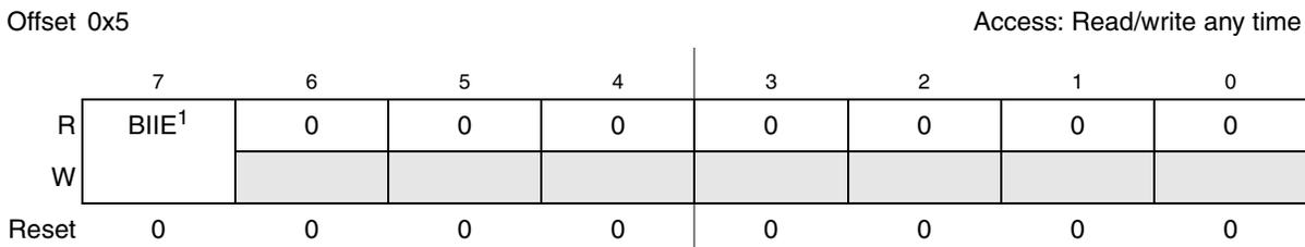
**Figure 22-9. I<sup>2</sup>C Bus Interrupt Config Register (IBIC)**
