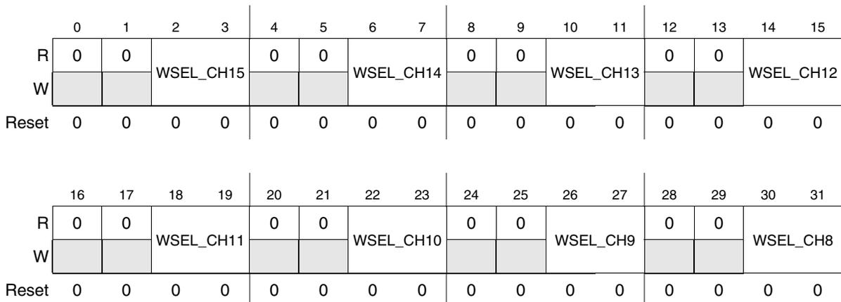
**Figure 28-61. Channel Watchdog Select Register 1 (CWSELR1) – ADC\_1**
