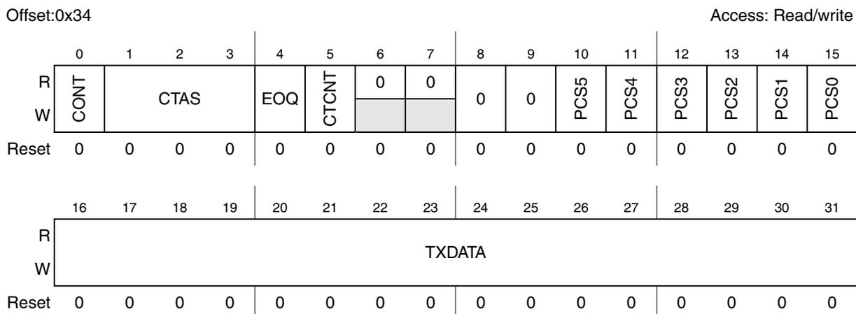
**Figure 26-8. DSPI PUSH TX FIFO Register (DSPIx\_PUSHR)**
