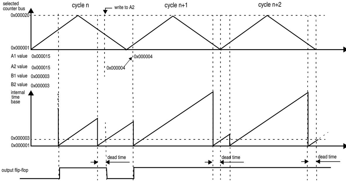
**Figure 27-43. OPWMCB with 100% Duty Cycle (A1 = 4 and B1 = 3)**
