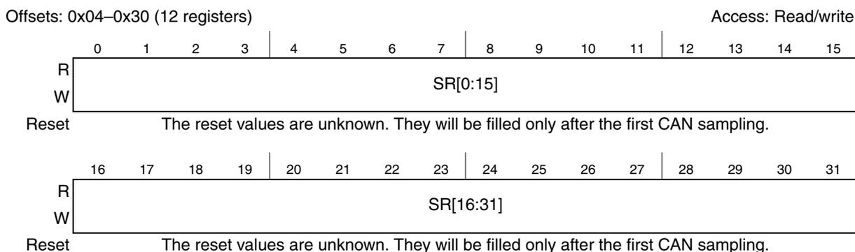
**Figure 14-3. CAN Sampler Sample Registers 0–11**
