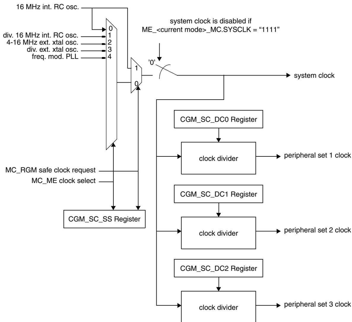
Figure 7-6. MC\_CGM System Clock Generation Overview
