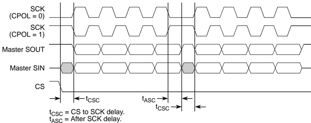
**Figure 26-21. Example of continuous transfer ( $CPHA = 1$ ,  $CONT = 1$ )**
