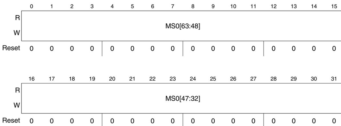
Figure 30-17. CFlash User Multiple Input Signature Register 1 (CFLASH\_UMISR1)
