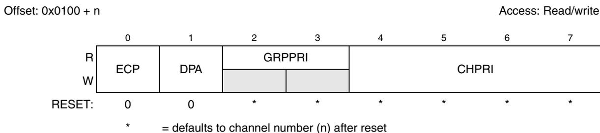
**Figure 16-17. DMA Channel n Priority (EDMA\_CPRn) Register**
