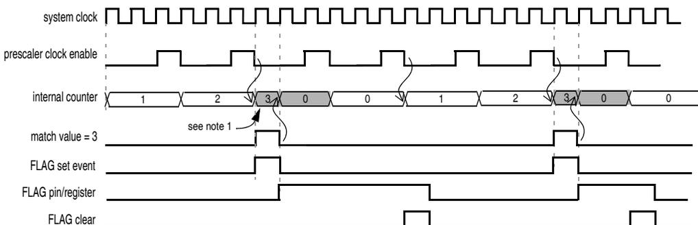
Note 1: When a match occurs, the first clock cycle is used to clear the internal counter, and only after a second edge of pre scaled clock the counter will start counting.
