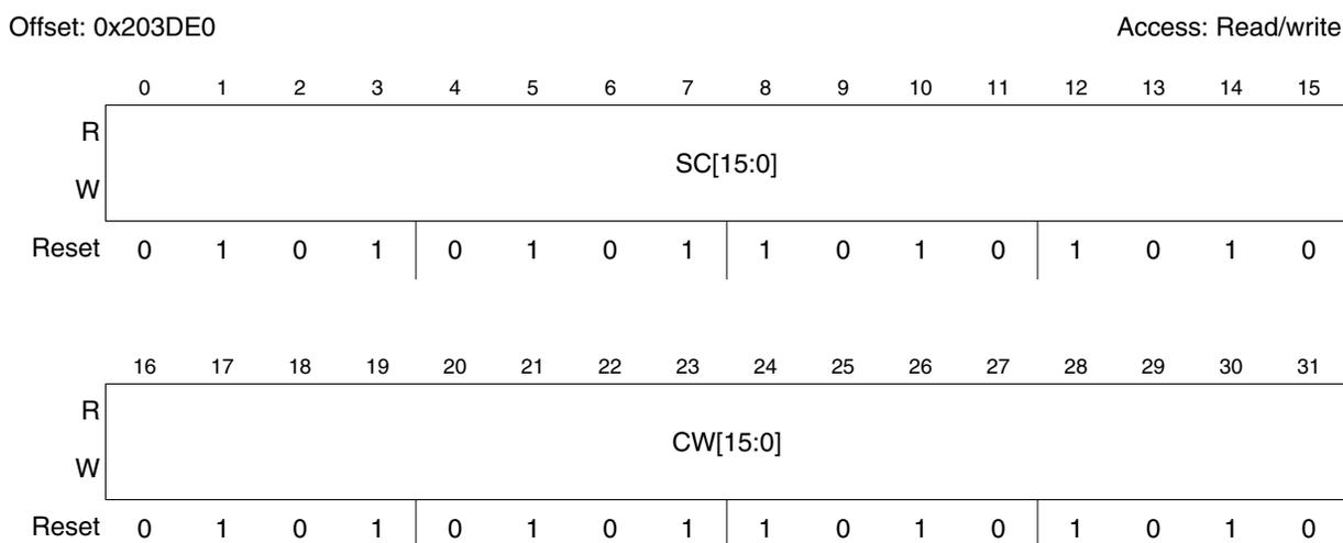
**Figure 30-23. CFlash Nonvolatile System Censorship Control 0 register (NVSCC0)**
