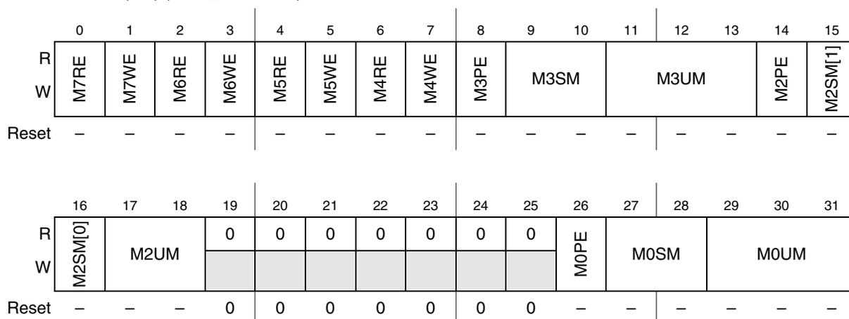
**Figure 20-9. MPU RGD Alternate Access Control n (MPU\_RGDAACn)**
