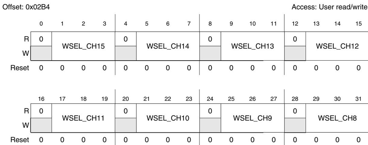
**Figure 28-51. Channel Watchdog Select Register 1 (CWSELR1) – ADC\_0**
