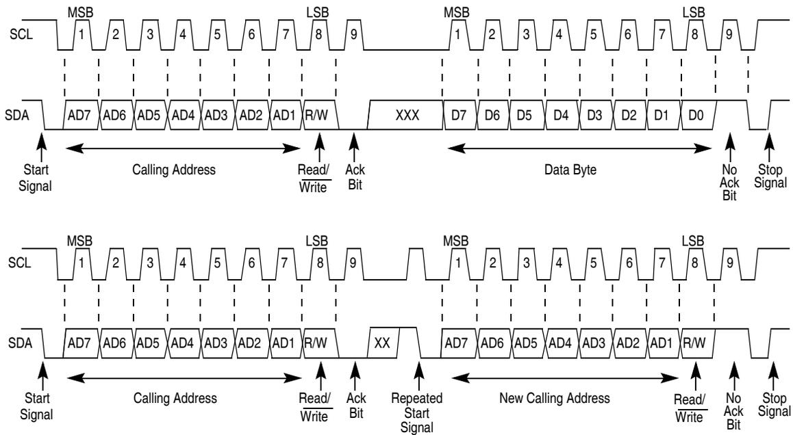
Figure 22-11. I<sup>2</sup>C bus transmission signals
