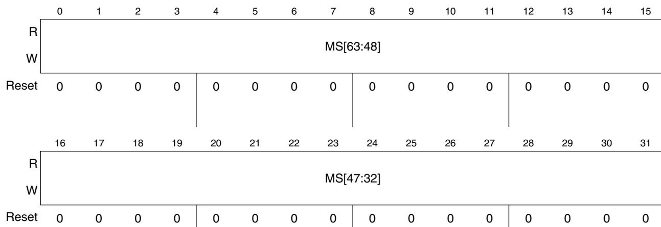
**Figure 30-37. DFlash User Multiple Input Signature Register 1 (DFLASH\_UMISR1)**
