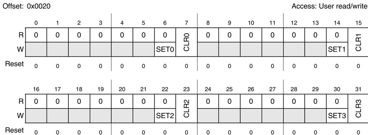
**Figure 18-7. INTC Software Set/Clear Interrupt Register 0–3 (INTC\_SSCIR[0:3])**
