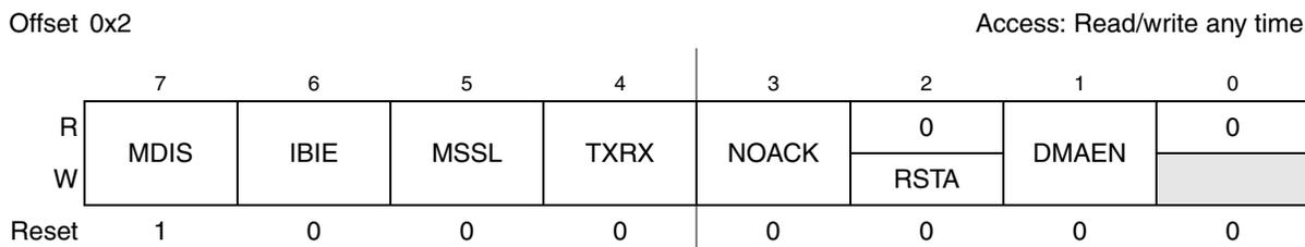
Figure 22-6. I<sup>2</sup>C Bus Control Register (IBCR)
