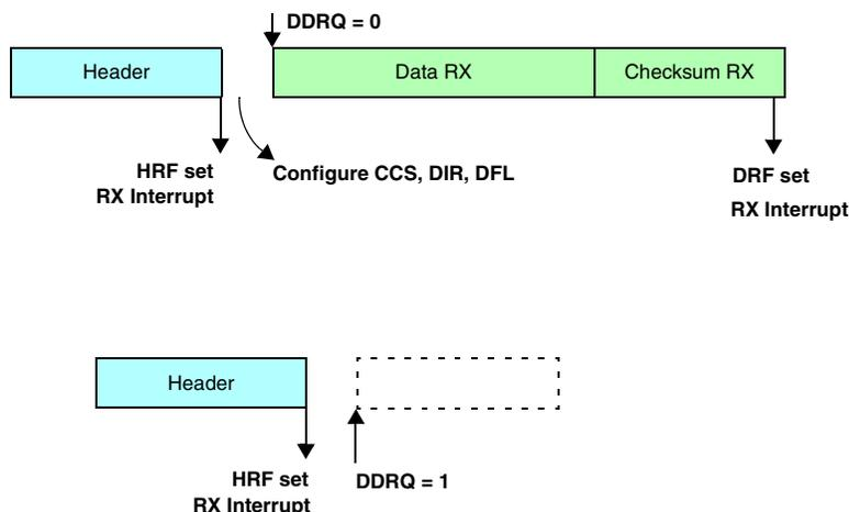
Figure 24-62. Programming consideration: slave node, receiver, no filters
