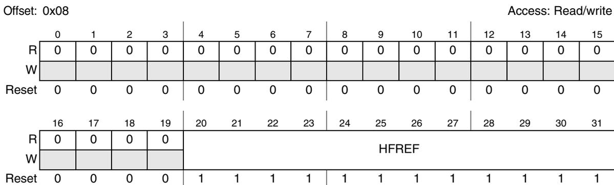
Figure 6-14. High Frequency Reference Register FMPLL (CMU\_HFREFR)
