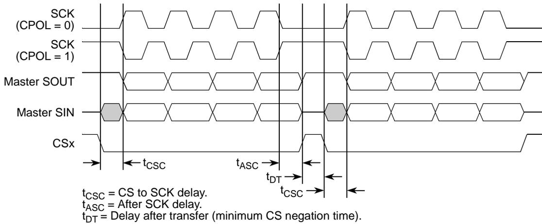
**Figure 26-20. Example of non-continuous format ( $CPHA = 1$ ,  $CONT = 0$ )**
