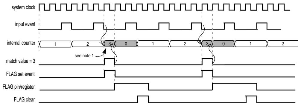
Note 1: When a match occurs, the first system clock cycle is used to clear the internal counter, and at the next edge of prescaler clock enable the counter will start counting.
