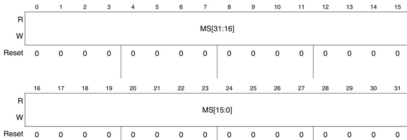
Figure 30-36. DFlash User Multiple Input Signature Register 0 (DFLASH\_UMISR0)
