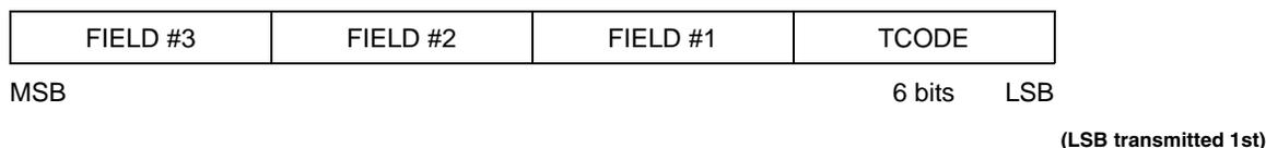
**Figure 36-7. Transmission Sequence of Messages**
