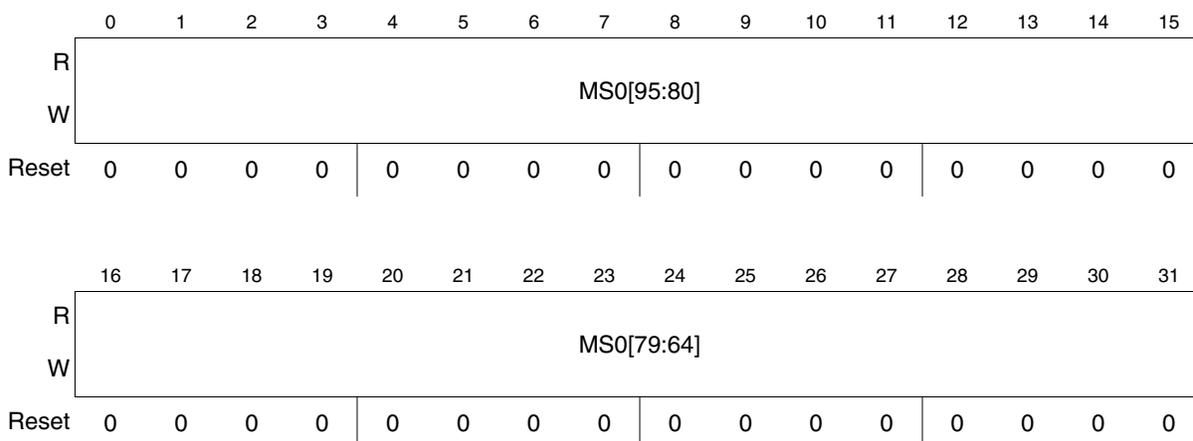
**Figure 30-18. CFlash User Multiple Input Signature Register 2 (CFLASH\_UMISR2)**
