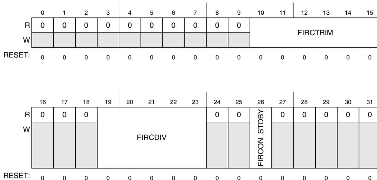
**Figure 6-5. FIRC Oscillator Control Register (FIRC\_CTL)**
