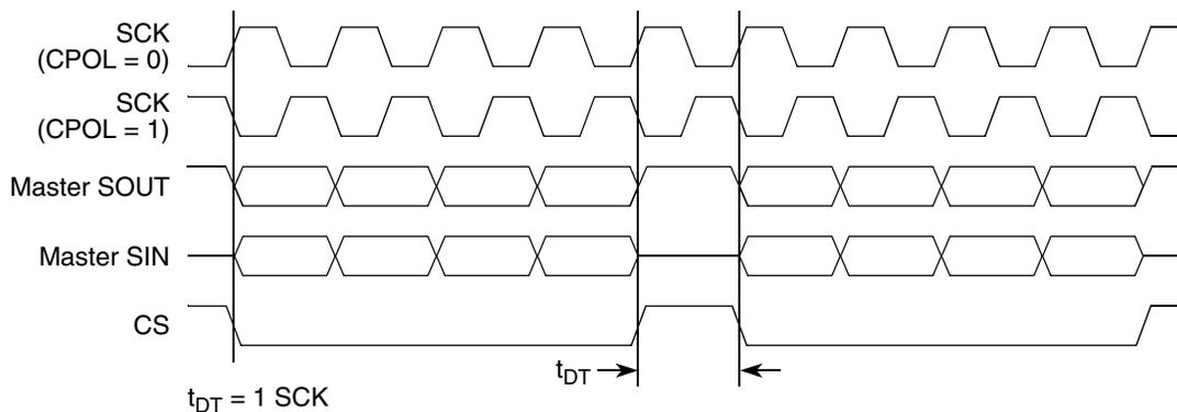
**Figure 26-23. Continuous SCK timing diagram (CONT= 0)**
