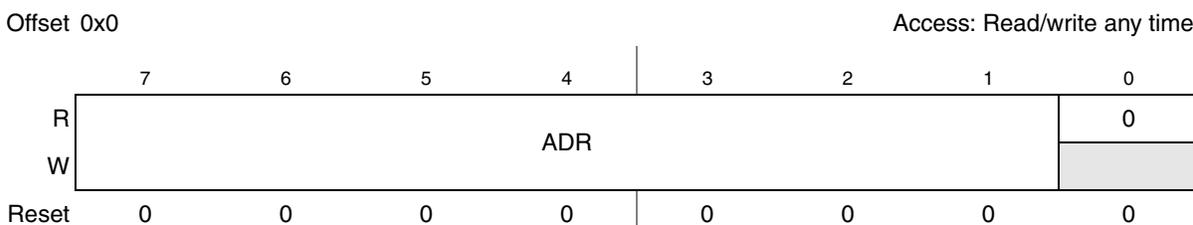
**Figure 22-2. I<sup>2</sup>C Bus Address Register (IBAD)**
