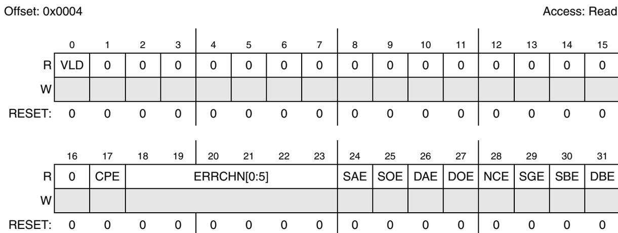
**Figure 16-3. DMA Error Status (EDMA\_ESR) Register**
