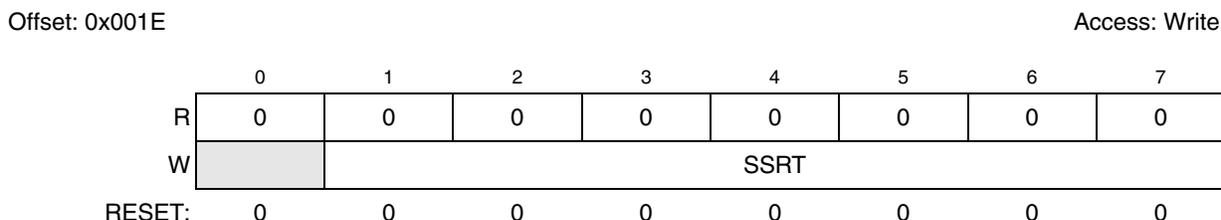
**Figure 16-12. DMA Set START Bit (EDMA\_SSBR) Register**
