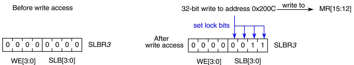
**Figure 32-10. Enable Locking for Protected and Unprotected Addresses**
