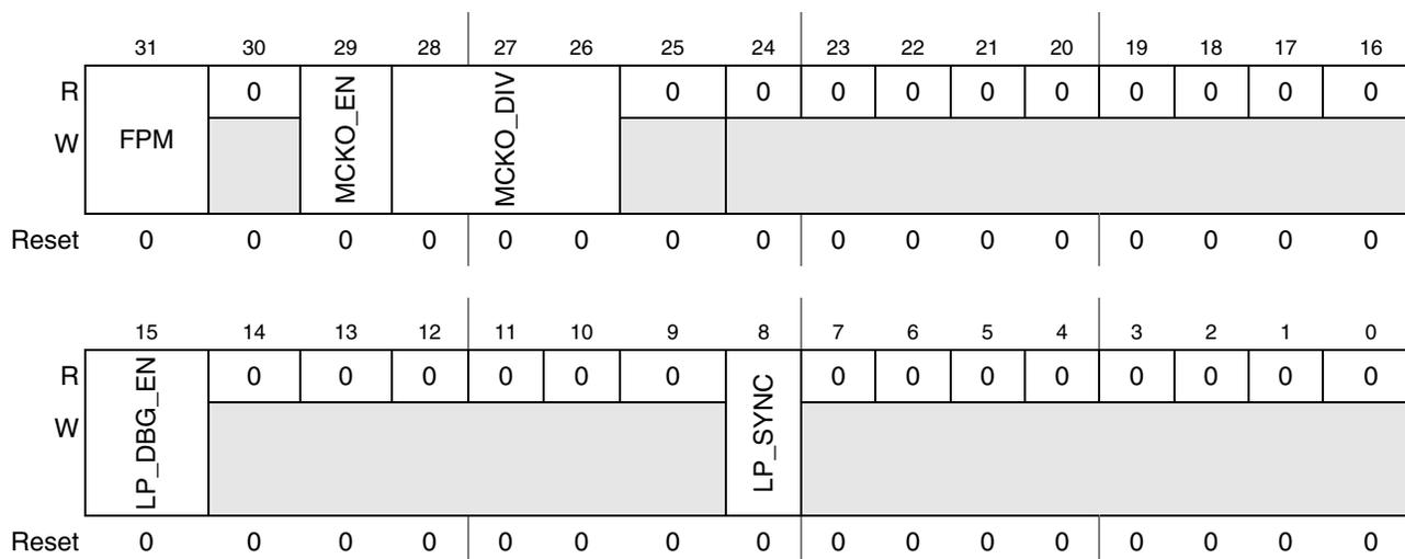
Figure 36-4. Port Configuration Register (PCR)
