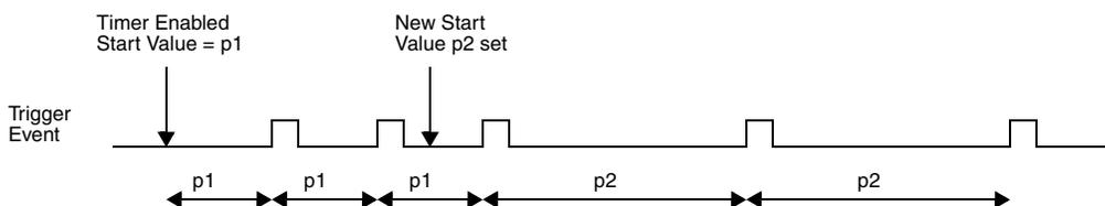
Figure 27-64. Dynamically setting a new load value
