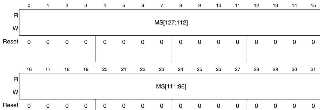
Figure 30-39. DFlash User Multiple Input Signature Register 3 (DFLASH\_UMISR3)
