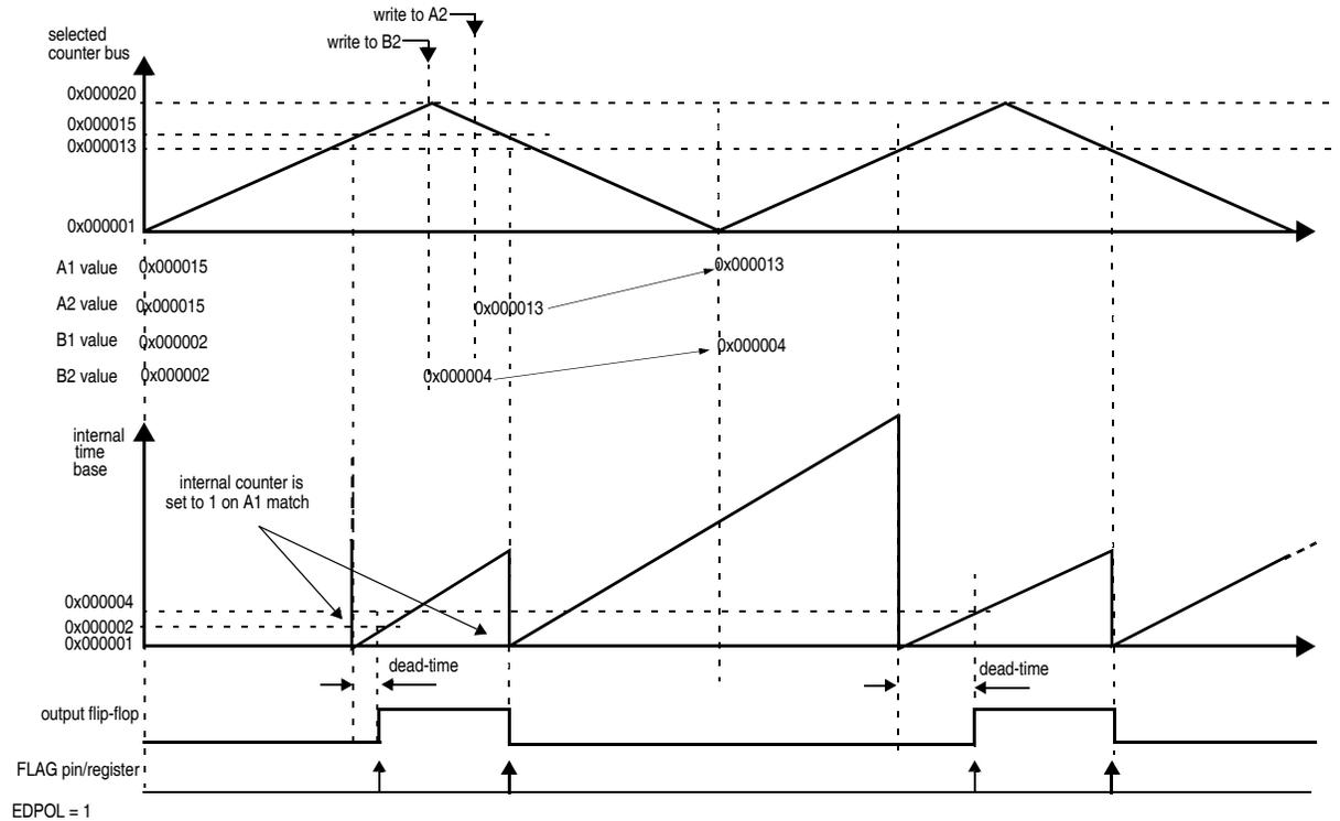
**Figure 27-41. OPWMCB with lead dead time insertion**
