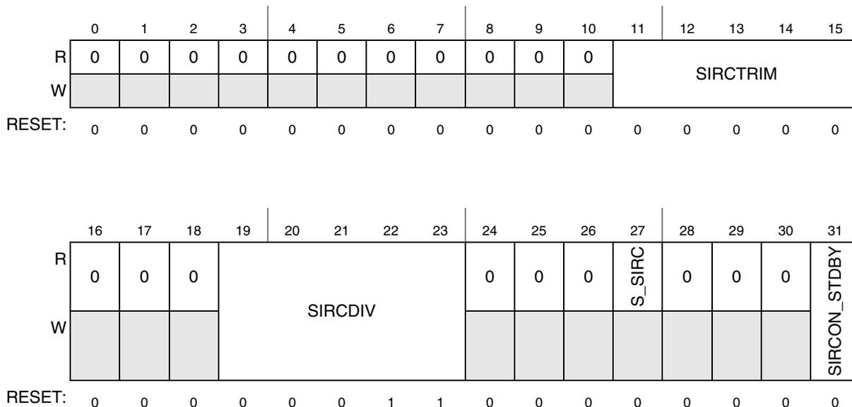
**Figure 6-4. Low Power RC Control Register (SIRC\_CTL)**
