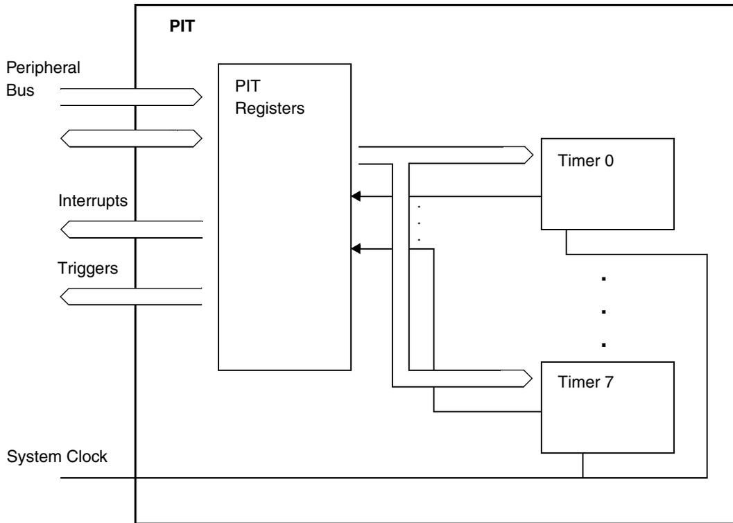
Figure 27-56. PIT block diagram
