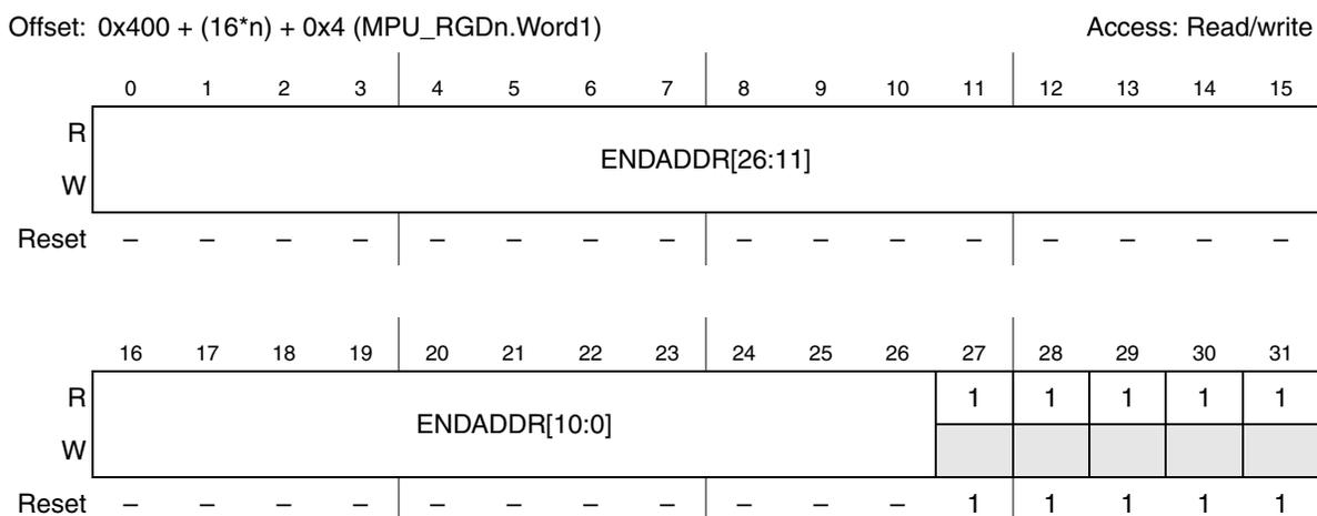
**Figure 20-6. MPU Region Descriptor, Word 1 Register (MPU\_RGDn.Word1)**
