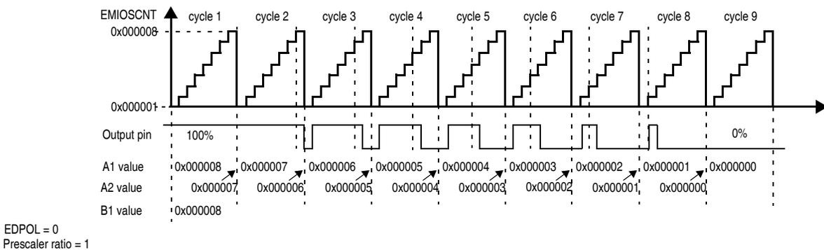
**Figure 27-39. OPWFMB mode from 100% to 0% duty cycle**
