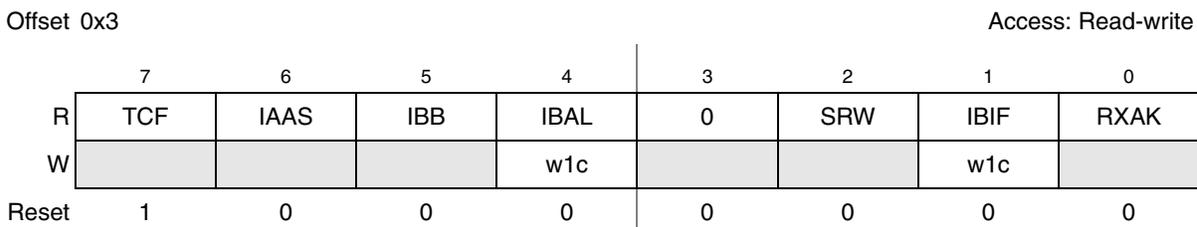
**Figure 22-7. I<sup>2</sup>C Bus Status Register (IBSR)**
