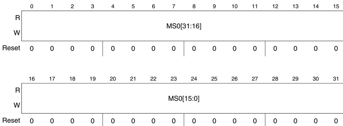
**Figure 30-16. CFlash User Multiple Input Signature Register 0 (CFLASH\_UMISR0)**
