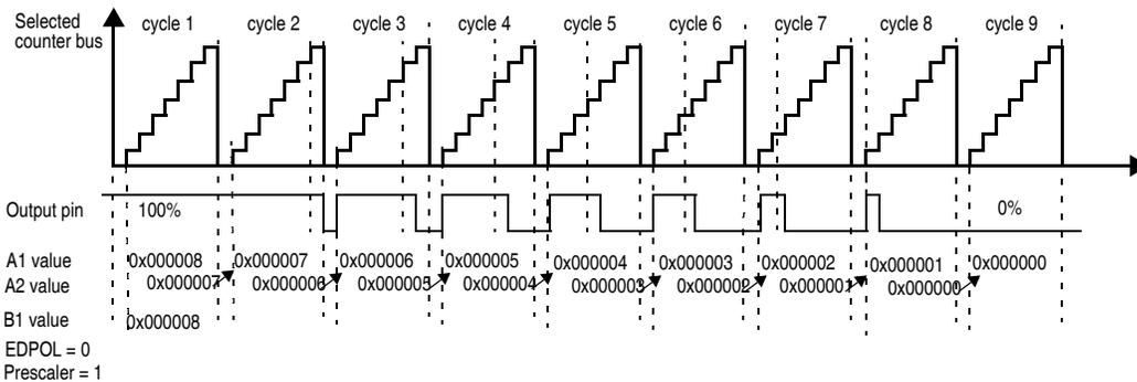
Figure 27-46. OPWMB mode from 100% to 0% duty cycle
