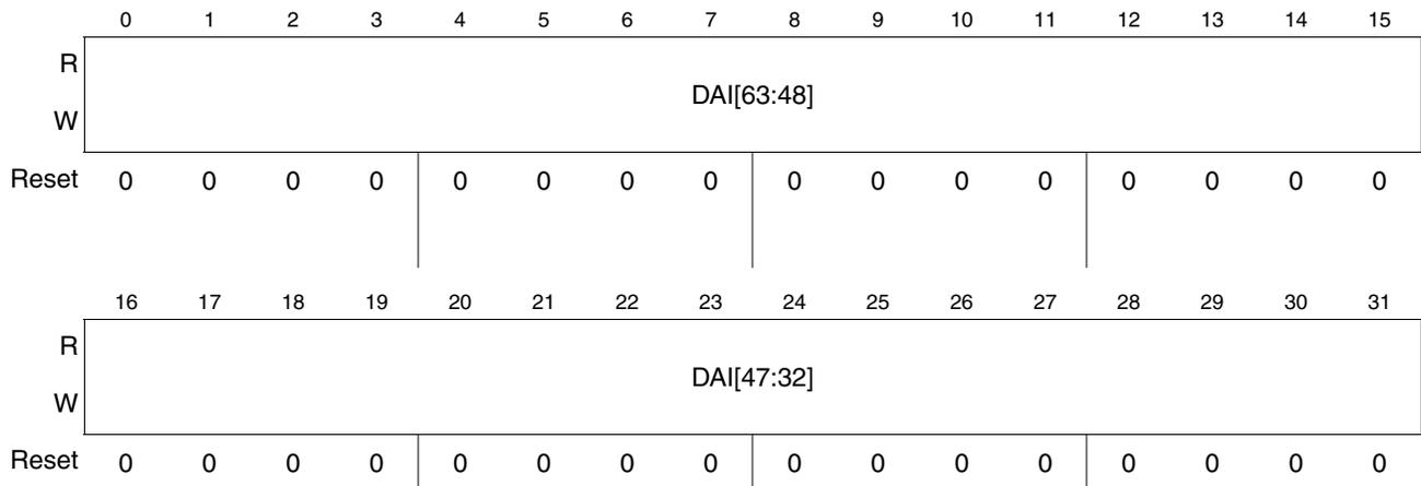
Figure 30-35. DFlash User Test 2 register (DFLASH\_UT2)
