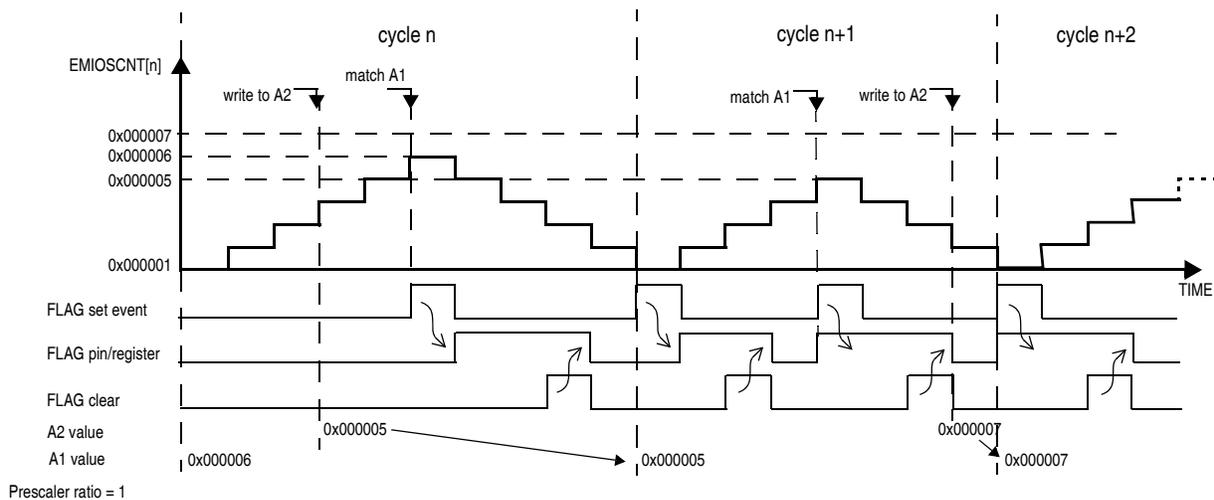
**Figure 27-33. Modulus Counter Buffered (MCB) Up/Down mode**
