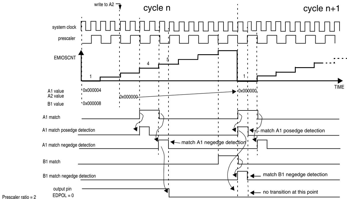
**Figure 27-37. OPWFMB Mode with A1 = 0 (0% duty cycle)**
