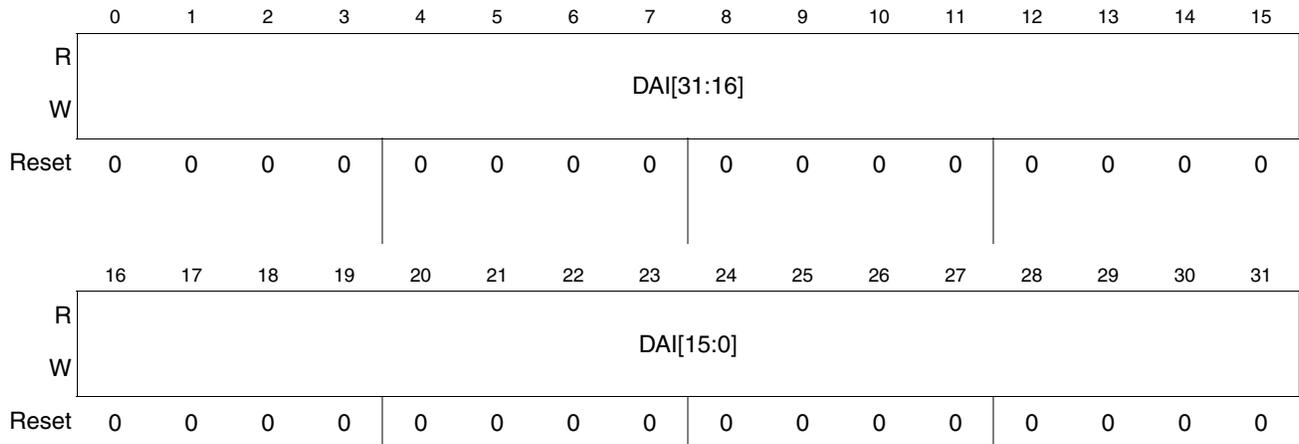
Figure 30-34. DFlash User Test 1 register (DFLASH\_UT1)
