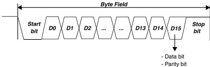
Figure 24-16. UART mode 16-bit data frame
