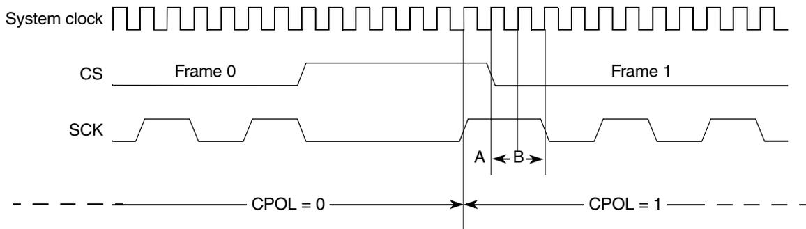
**Figure 26-22. Polarity switching between frames**
