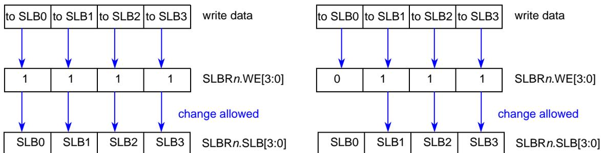
Figure 32-5. Change Lock Settings Directly Via Area #4
