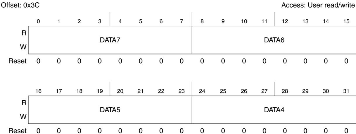
**Figure 24-33. Buffer data register most significant (BDRM)**
