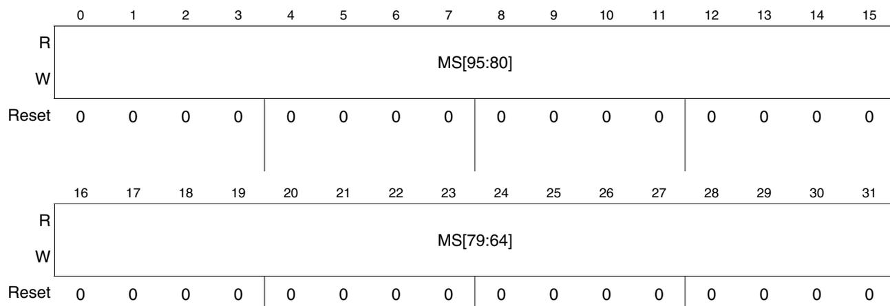
Figure 30-38. DFlash User Multiple Input Signature Register 2 (DFLASH\_UMISR2)
