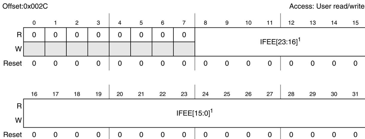
**Figure 21-7. Interrupt Falling-Edge Event Enable Register (IFEER)**
