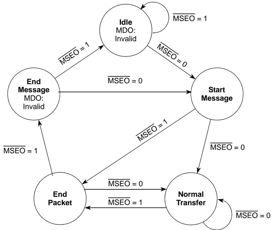
Figure 36-5.  $\overline{\text{MSEO}}$  Transfers
