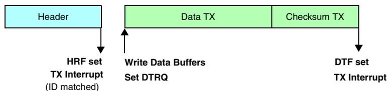
**Note:** This configuration can be used in case the slave never receives data (for example, as with a sensor).
