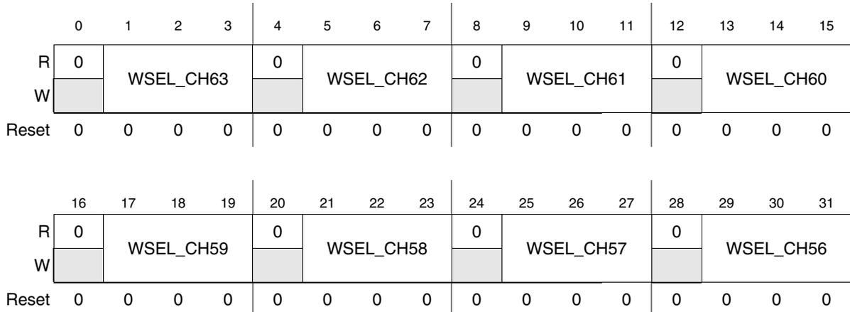
**Figure 28-55. Channel Watchdog Select Register 7 (CWSELR7) – ADC\_0**
