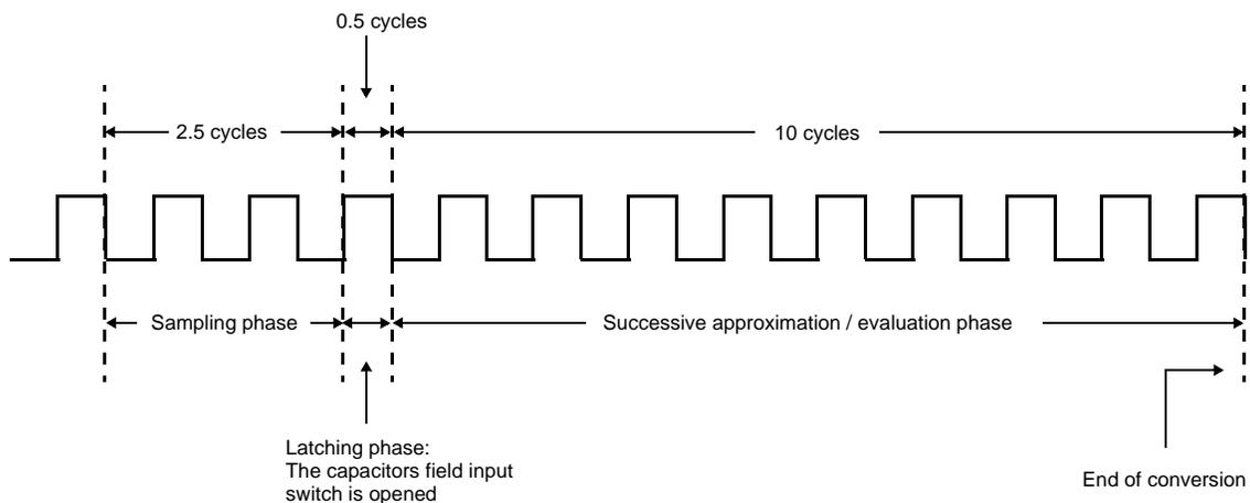
**Note:** Operating conditions — INPLATCH = 0, INPSAMP = 3, INPCMP = 1 and Fadc clk = 20 MHz
