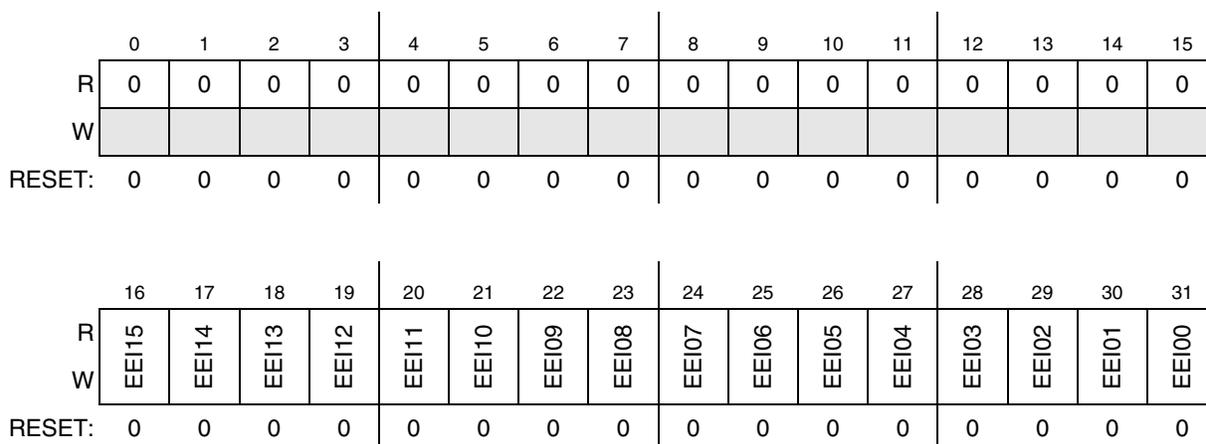
Figure 16-5. DMA Enable Error Interrupt (EDMA\_EEIRL) Register
