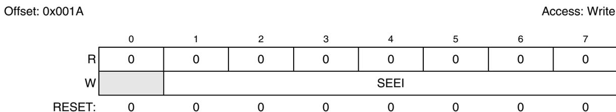
**Figure 16-8. DMA Set Enable Error Interrupt (EDMA\_SEEIR) Register**
