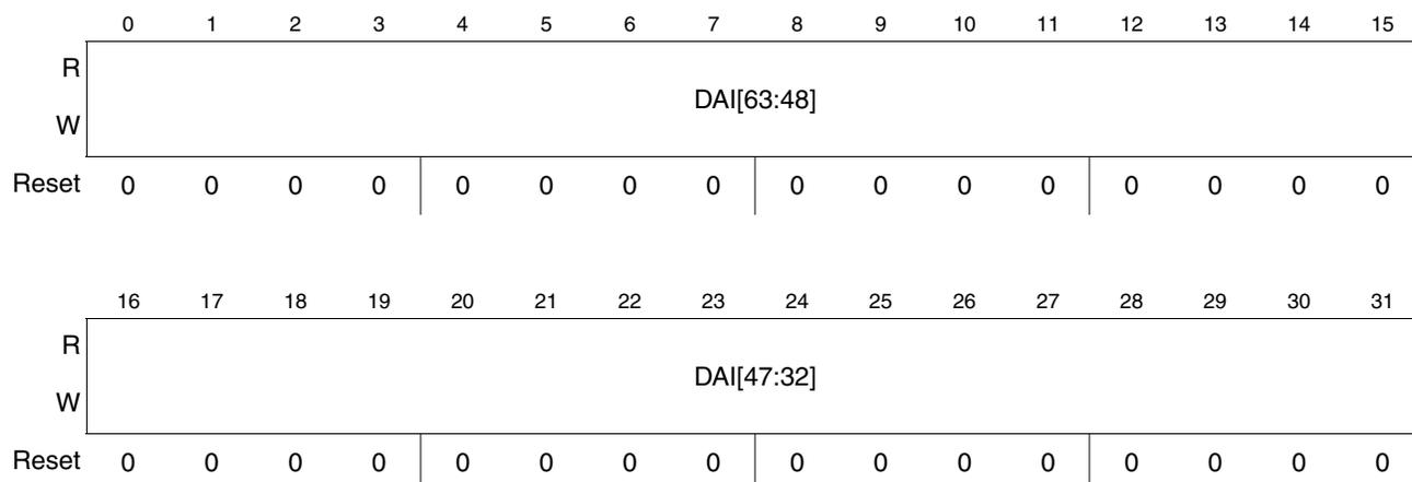
Figure 30-15. CFlash User Test 2 register (CFLASH\_UT2)
