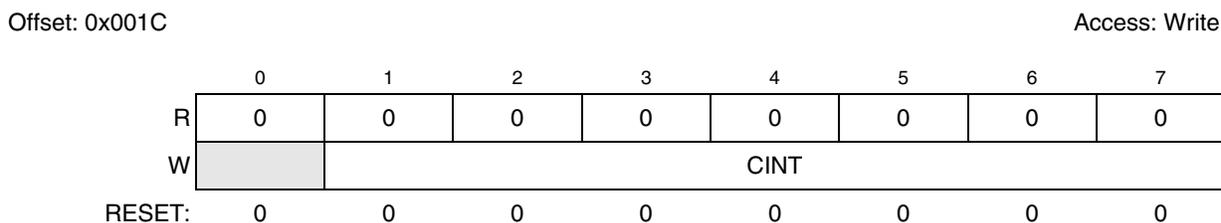
**Figure 16-10. DMA Clear Interrupt Request (EDMA\_CIRQR) Fields**
