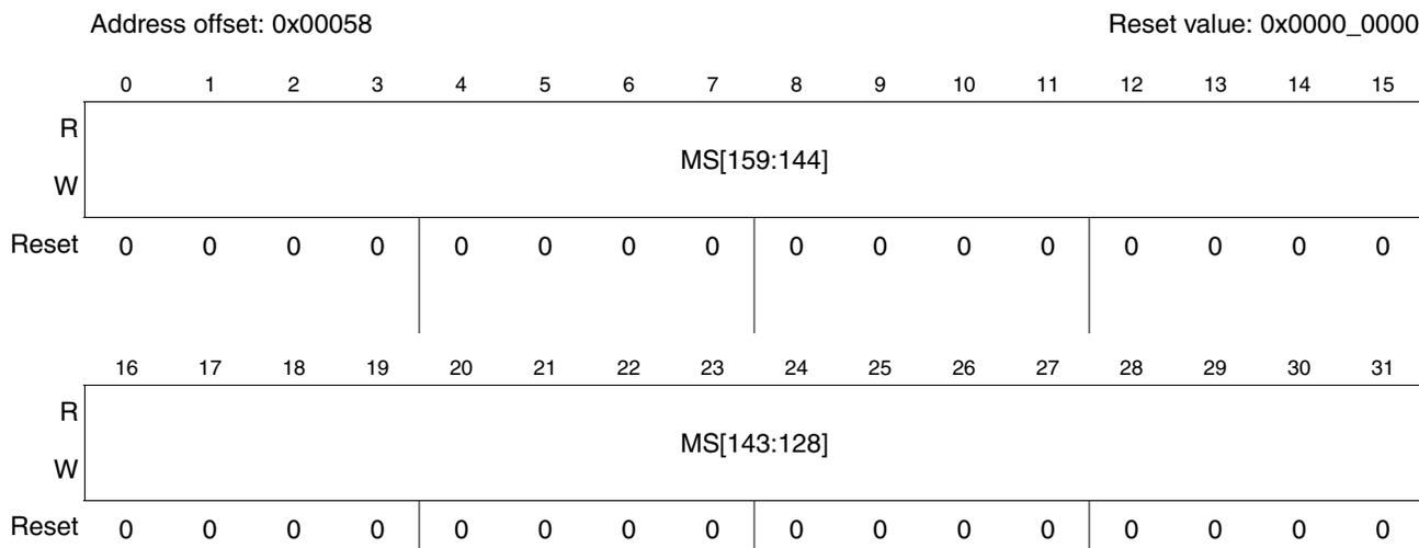
**Figure 30-40. DFlash User Multiple Input Signature Register 4 (DFLASH\_UMISR4)**
