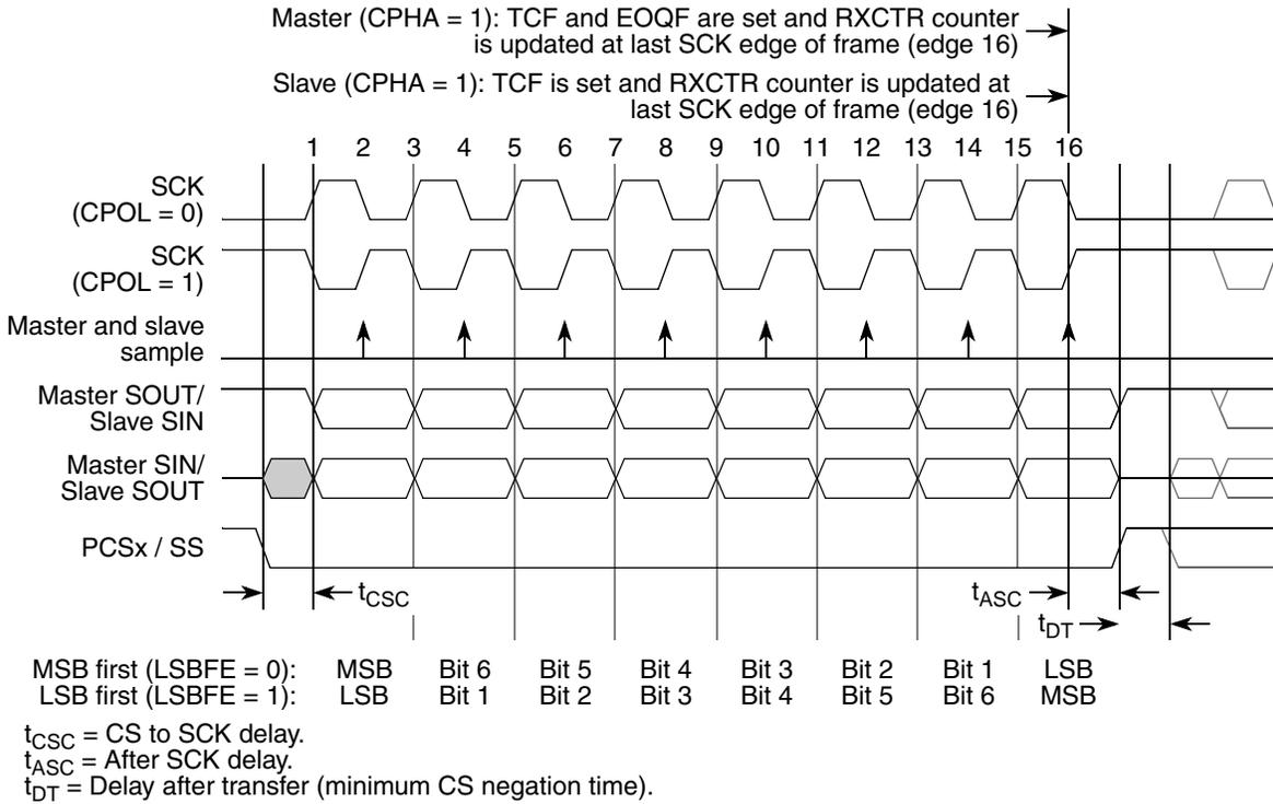
Figure 26-17. DSPI transfer timing diagram (MFE = 0, CPHA = 1, FMSZ = 8)
