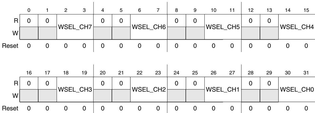
**Figure 28-60. Channel Watchdog Select Register 0 (CWSELR0) – ADC\_1**
