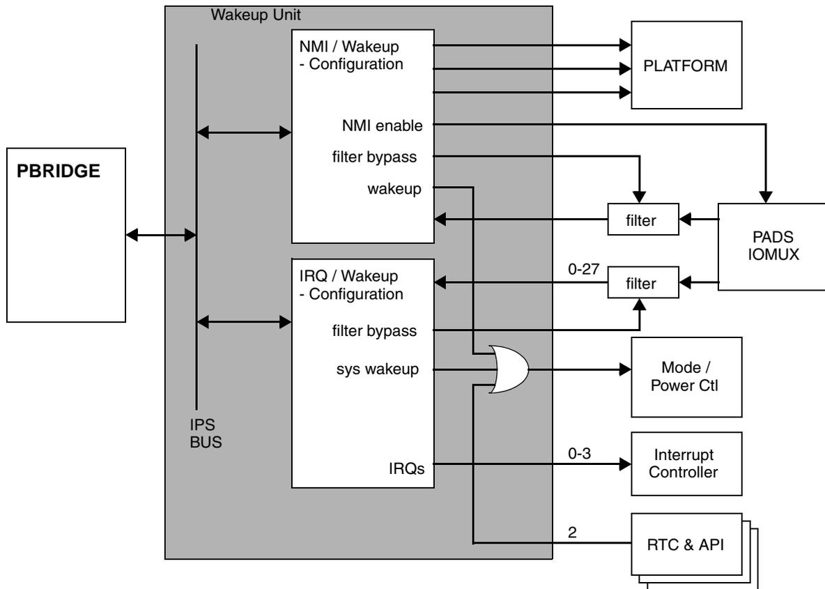
Figure 12-1. WKPU block diagram
