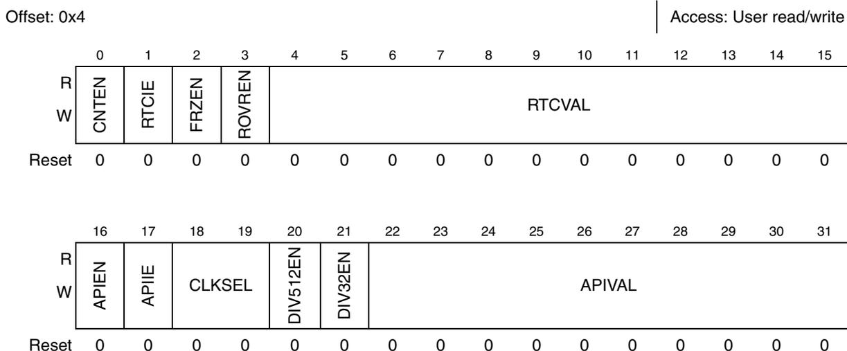
**Figure 13-4. RTC Control Register (RTCC)**
