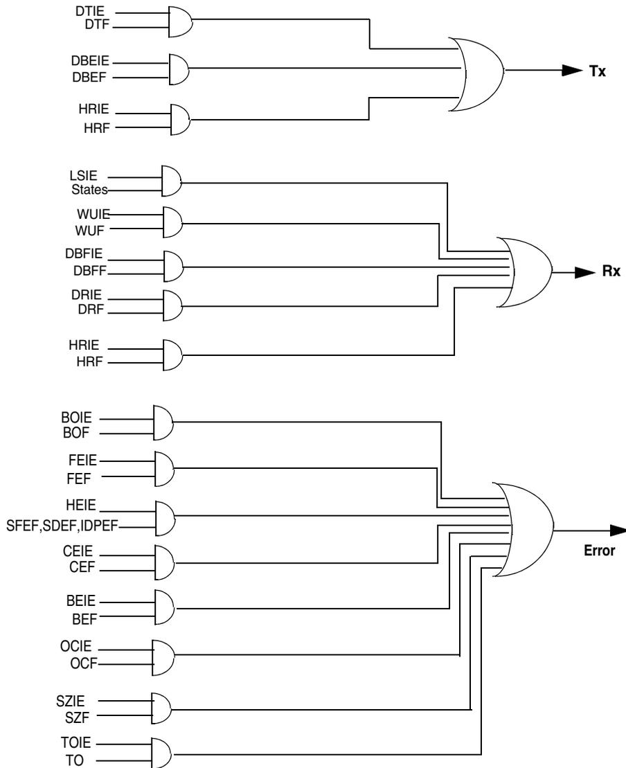
Figure 24-56. Interrupt diagram
