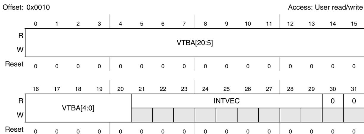
**Figure 18-4. INTC Interrupt Acknowledge Register (INTC\_IACKR) when INTC\_MCR[VTES] = 0**
