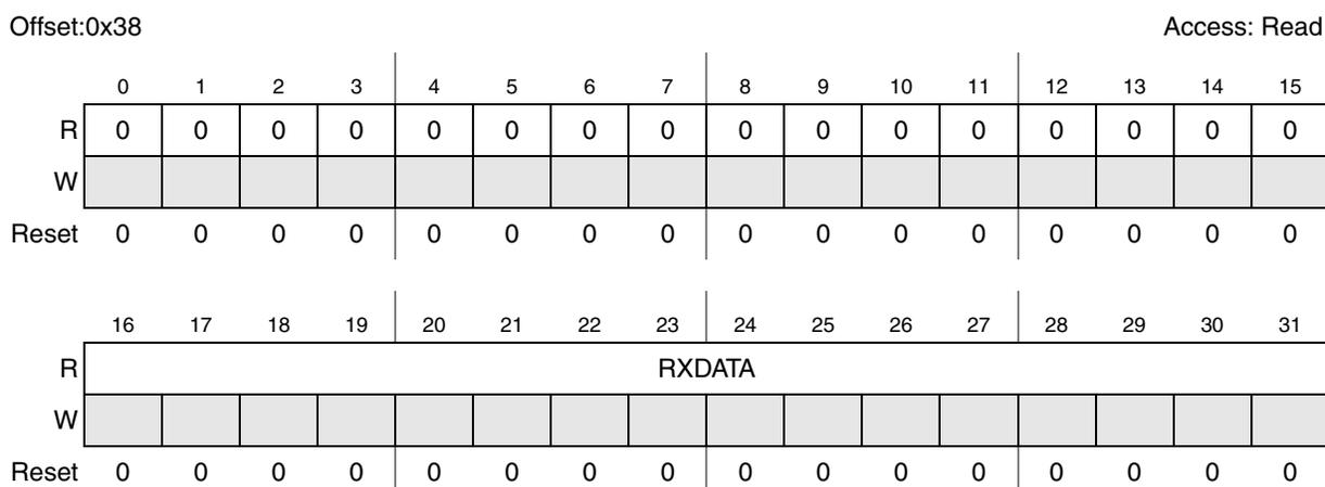
**Figure 26-9. DSPI POP RX FIFO Register (DSPIx\_POPR)**
