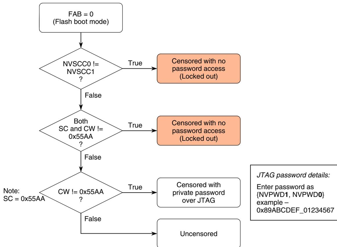
Figure 5-4. Censorship control in flash memory boot mode
