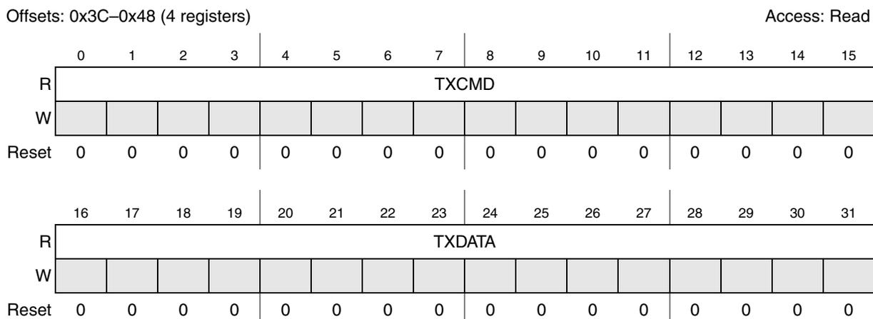
Figure 26-10. DSPI Transmit FIFO Register 0–3 (DSPIx\_TXFRn)
