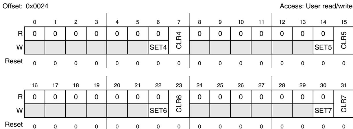
**Figure 18-8. INTC Software Set/Clear Interrupt Register 4–7 (INTC\_SSCIR[4:7])**
