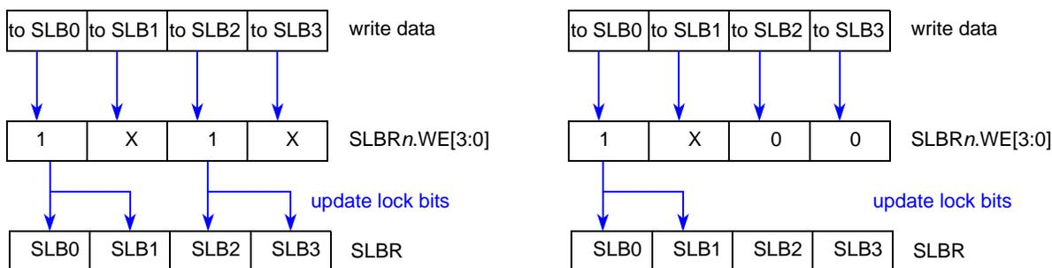
Figure 32-6. Change Lock Settings for 16-bit Protected Addresses
