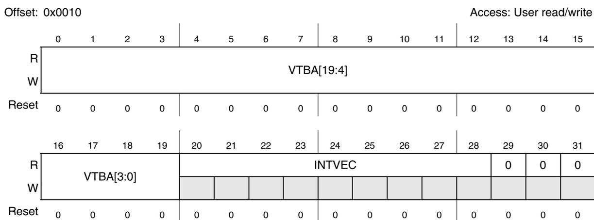
**Figure 18-5. INTC Interrupt Acknowledge Register (INTC\_IACKR) when INTC\_MCR[VTES] = 1**
