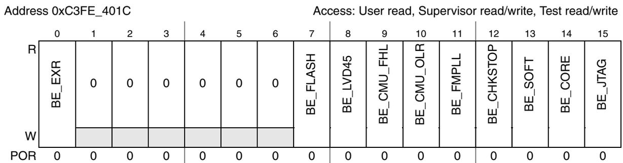
Figure 9-10. Functional Bidirectional Reset Enable Register (RGM\_FBRE)
