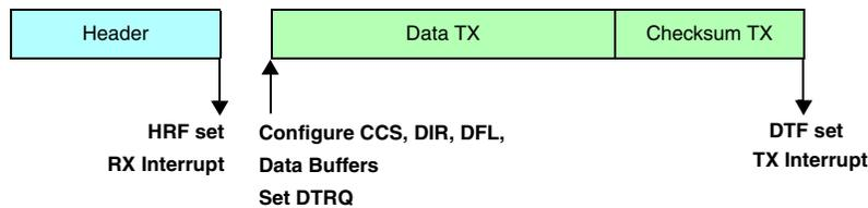
Figure 24-61. Programming consideration: slave node, transmitter, no filters
