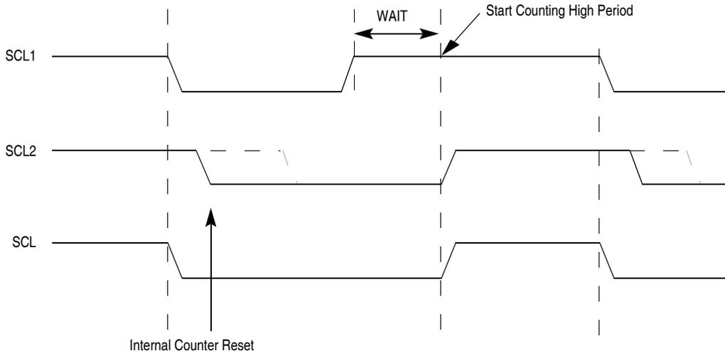
Figure 22-13. I<sup>2</sup>C bus clock synchronization
