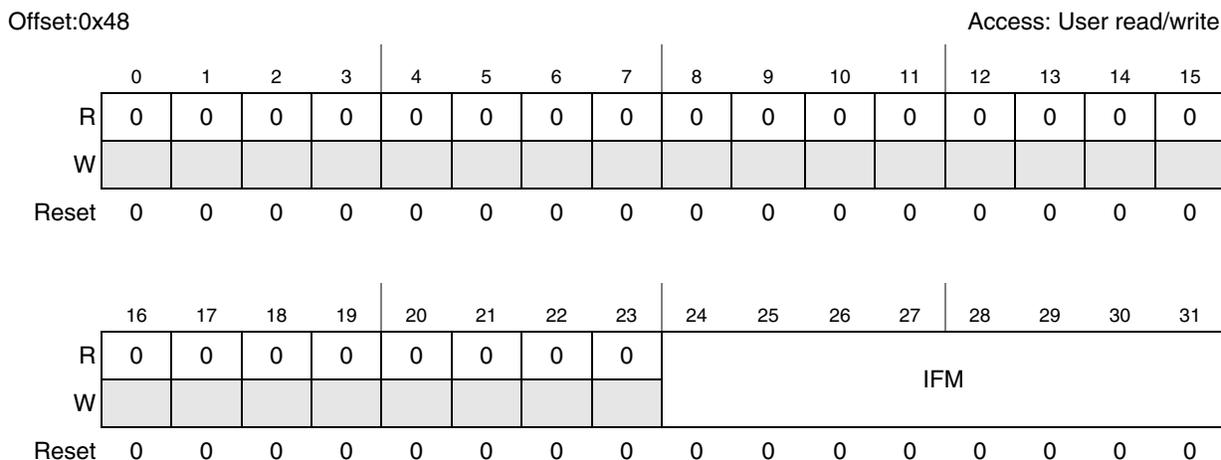
**Figure 24-36. Identifier filter mode register (IFMR)**
