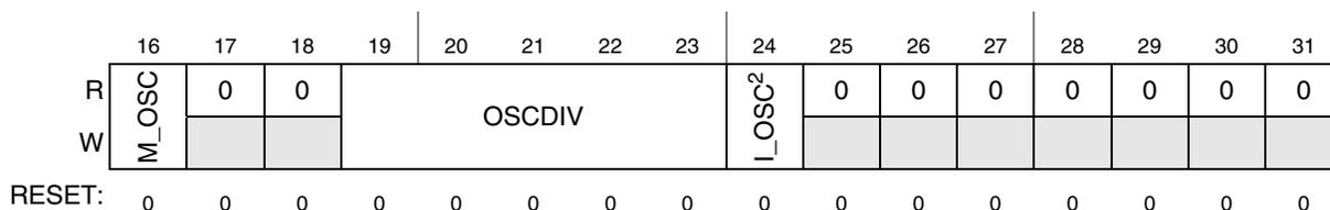
**Figure 6-2. Fast External Crystal Oscillator Control Register (FXOSC\_CTL)**
