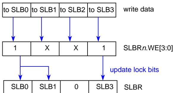
**Figure 32-8. Change Lock Settings for Mixed Protection**
