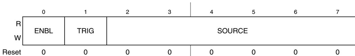
**Figure 17-2. Channel Configuration Registers (CHCONFIG $n$ )**
