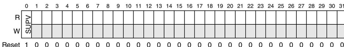
Figure 13-3. RTC Supervisor Control Register (RTCSUPV)
