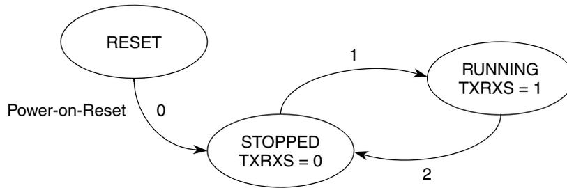
**Figure 26-13. DSPI start and stop state diagram**
