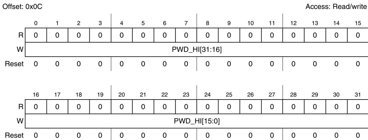
**Figure 5-17. Password Comparison Register High Word (SSCM\_PWCMPH)**
