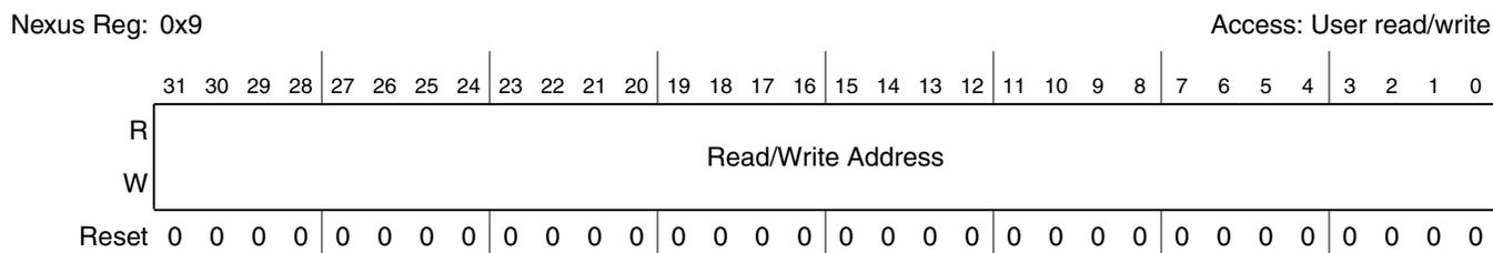
**Figure 36-15. Read/Write Access Address Register (RWA)**
