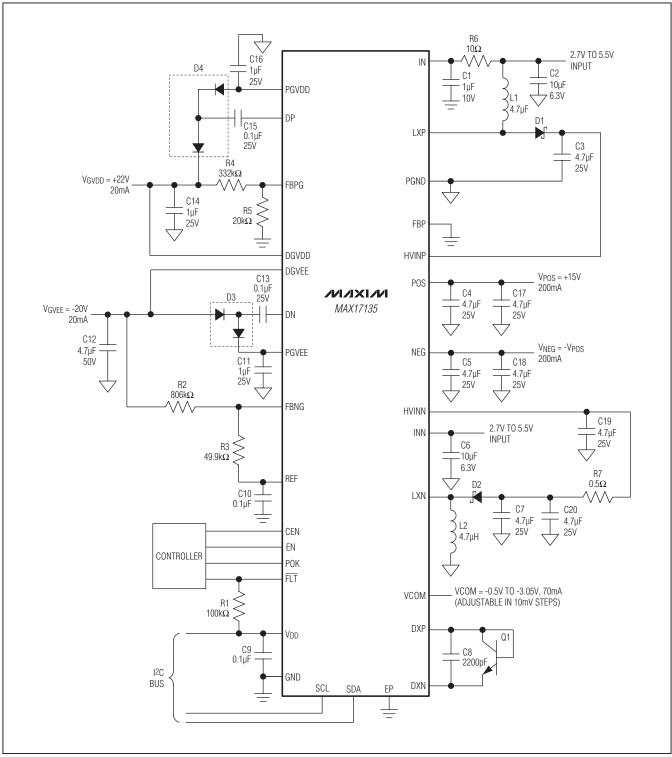
Figure 2. Typical Operating Circuit
