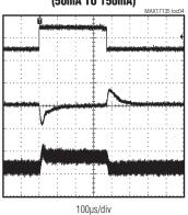
IPOS 100mA/div 0mA VPOS (AC-COUPLED) 100mV/div 0mV ILX1 1A/div 0A VIN = 3.6V
