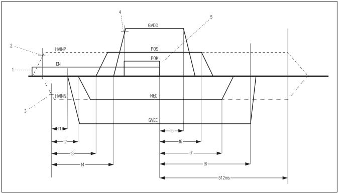
Figure 5. Adjustable Power-Up and Power-Down Sequencing
