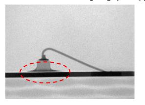
If the peak temperature is too high (excessive), it may cause delamination between Ag paste and circuit board due to warpage of printed wiring circuit board or expansion of resin. And if the temperature gradient of temperature rising/falling is large, it can also cause delamination, so please use it in  $1\sim3$ °C/sec.
