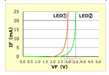
Therefore, 1 resistor per LED can reduce difference of current value to have uniform luminous intensity.
