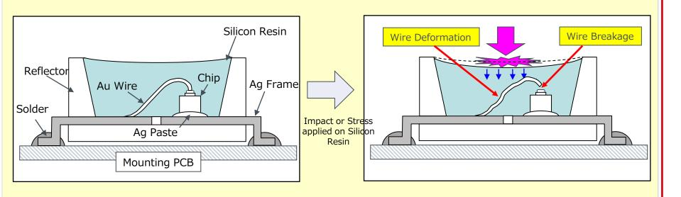
When it is mounting, please have the adsorption collet touching with reflector. After it is mounted, please be care to handle with the part of sealing.
