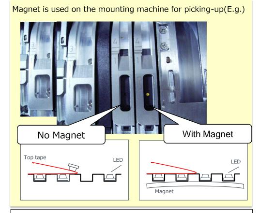
For super small products, it may paste on tape due to static electricity because of the operational environment. In the case, it can solve the problem by installing a magnet on the mounting machine.
