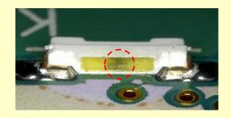
The Ag of frame is corroded and its color changed into black
