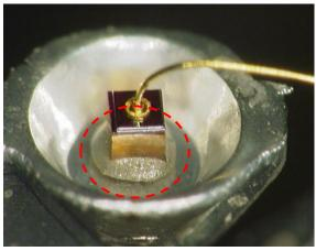
If the flow soldering condition is strict, it may cause the delamination of Ag-paste and frame due to over heat stress around the lead frame and die bonding.
