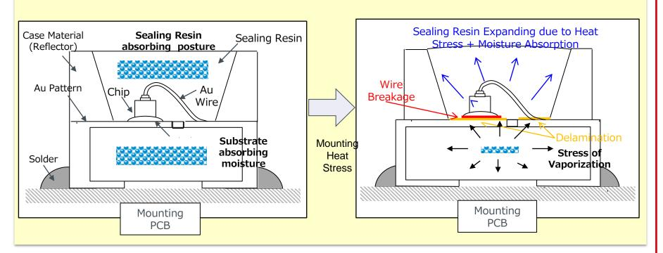
When the product is absorbing the moisture, the vaporized stream (by the heat of reflow)will go out, its stress will lift up the sealing resin from the bottom and result in breakage of wire bonding.
