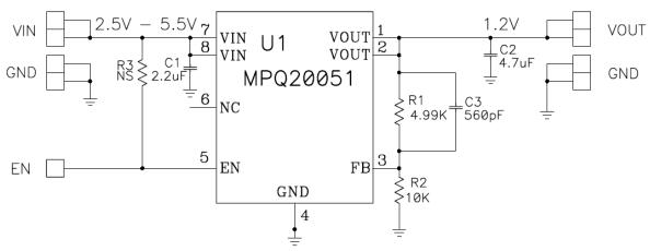
Figure 3: 1.2V Output Typical Application Schematic
